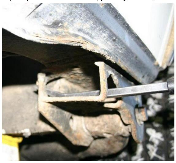
Hang the ladder from the rain gutter and screw the bump stop **OUT** until it just touches the body of your van.
