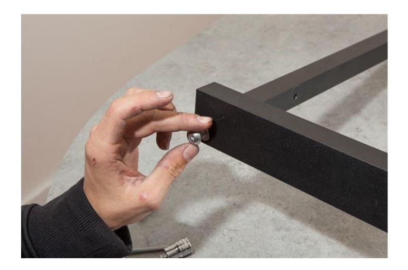
Use a 7/32" Hex Bit Socket and a Ratchet in order to tighten the Button Head Screw. DO NOT FULLY TIGHTEN AT THIS POINT. Leave a few threads shy of fully tightening. This will allow the installation of the Ladder Rungs to go more smoothly. Repeat the process for the opposite Upper Ladder Stringer as well.
