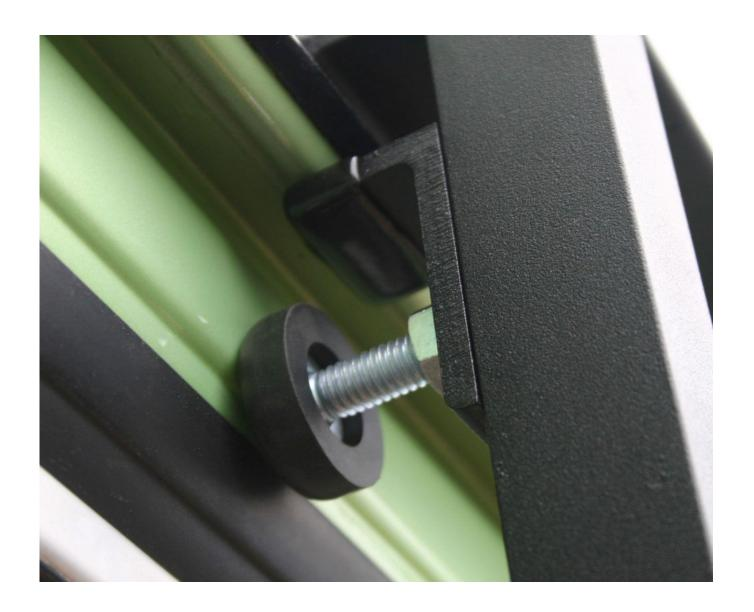
Move to the lower section and push the bottom of the ladder into the jack point until the hole for the second pin is inside the jack point. The ladder should now be under slight tension so it does not rattle or vibrate. If there is still looseness in the fit, screw the bump stop a little tighter against the body of the van. The goal is to have the ladder secure but not tightly sprung.
