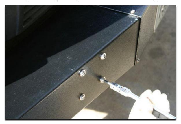
2. Once removed, set the appropriate pillar mount in place with the d-rings toward the outside of the van, and the pillar towards the middle.
