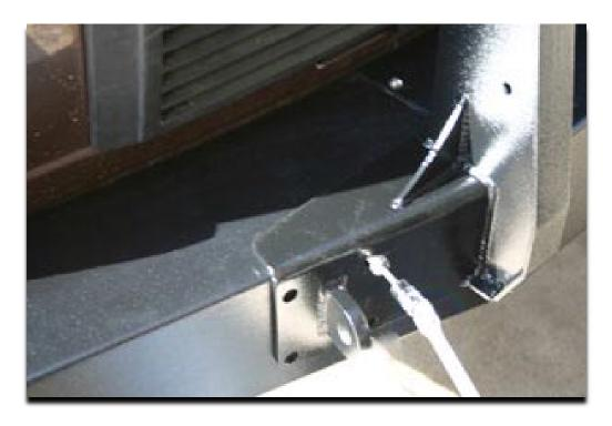
3. Using 4 - 3/8x16x1.25 SS button heads and 4- washers attach the pillar to the bumper. Using a small screwdriver or rod will help in keeping the pieces aligned. Do not fully tighten the pillars at this time.
