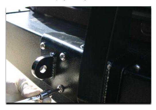
4. Slide the center frame section between the pillars. (At this point, 4 hands are better than two.) Start by inserting a 3/8x16x1.25 SS button head bolt with washer into the top hole of the appropriate side frame. Attach with a 3/8" lock nut and washer. Repeat for the rest of the holes. Install and set the other side frame in the same manner
