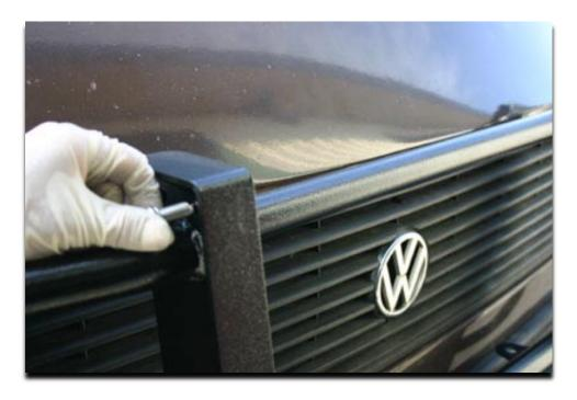
5. Tighten all frame bolts first, then the pillar bolts attached to your bumper.
