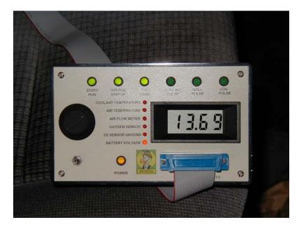
Now rotate the selector switch to the full counterclockwise position, COOLANT TEMPERATURE. This should illuminate the red coolant temperature indicator, and the digital display should indicate approximately .95 V. This value will depend on the coolant temperature at the time.
