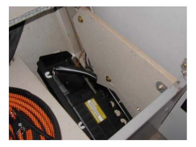
Now you need to remove the electrical connector from the ECU, in order to take the ECU black box out from the rear seat. Press on the small metal tab on the left side of the ECU itself. This will allow the electrical connector to be "hinged back" up and to the right like so:
