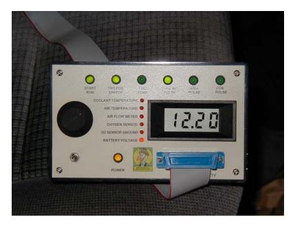
The green START/RUN, THROTTLE POSITION SWITCH, AND INJECTOR PULSE LEDs and the red BATTERY VOLTAGE LED should illuminate. The digital display should display approximately 12V.
