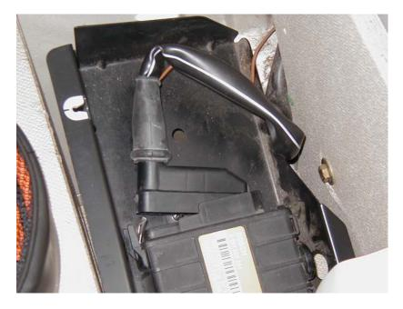
Now remount the ECU assembly back onto the right hand rear seat support. First, position the lower screw slot on the screw even with the bottom of the ECU black box. Once this is done, replace the two upper screws, making them snug, but NOT tight. Route the gray ribbon cable as shown, and lower the rear seat. Your test ECU is installed.
