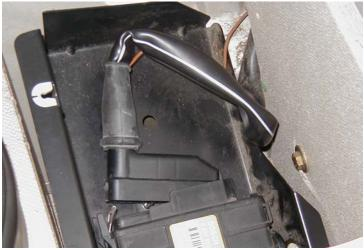
Now remove the electrical connector by swinging it up and to the right, removing the small tab from the opening at the right end of the connector socket.
