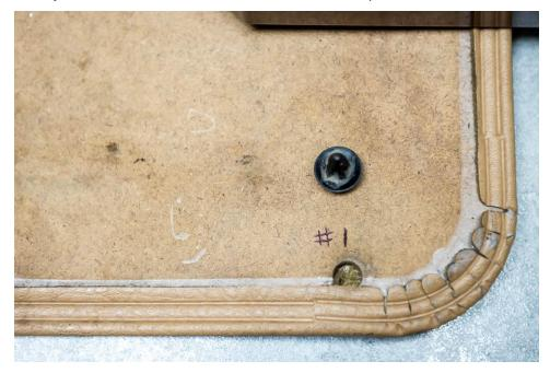
**Here are clips #2 and #3.** They're located along the bottom of the door panel near where the sliding vent was (you DID remove the vent, didn't you?).
