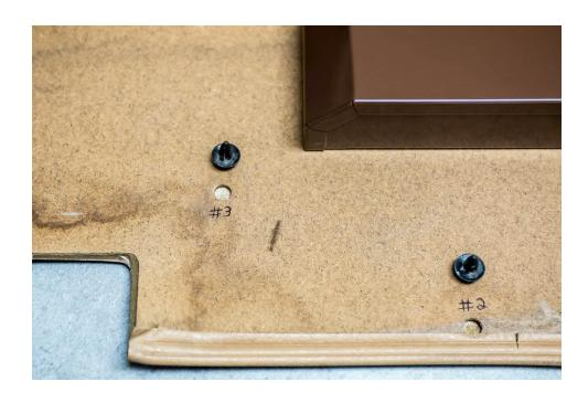
**STEP 5:** Cut out vinyl from holes #1 and #3 Take an exacto knife or other precision cutting blade and *carefully* cut out the vinyl from holes #1 and #3. Try and get as clean a cut as possible around the round hole.
