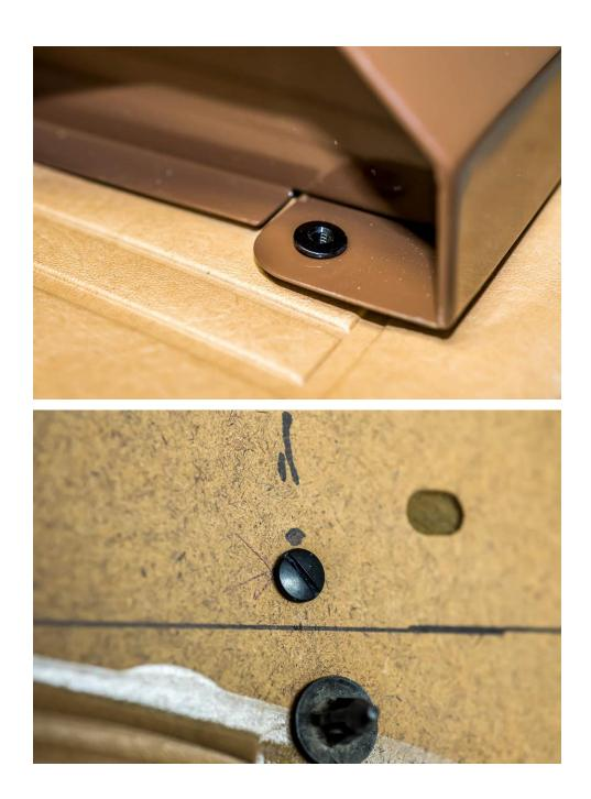
**STEP 12:** Reinstall the door panels Take one of the panel clips you removed way back at the beginning of this project and, from the back side of the panel, twist it back into hole #2. You now need to lengthen your speaker wires approximately 3-4" in order to install the speakers in your fancy new pockets. Do so now, we'll wait..... Got that finished? Great!
