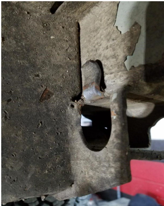
Figure 4: ...flatten it up against the inside of the jack point.
