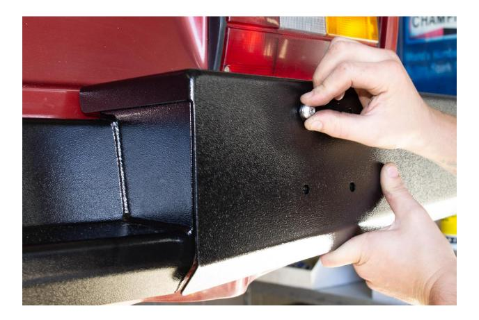
15. Remember that when installing a component with multiple fasteners, get all the fasteners started in their threads before you begin tightening. Tighten hardware evenly.
