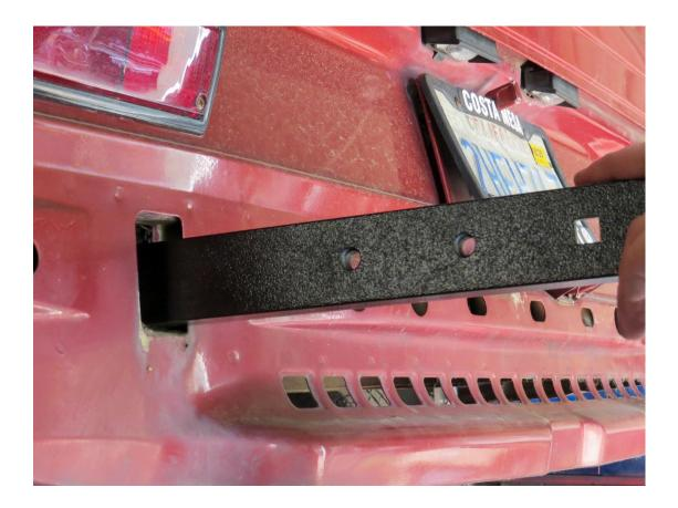
4. Insert an M12 hex bolt through a washer and start the bolt into the bracket from the outside of the frame rail. Leave all bolts loose until all three are in place and then tighten to 33 ft/lbs. Repeat on other side of Van with the second bracket.
