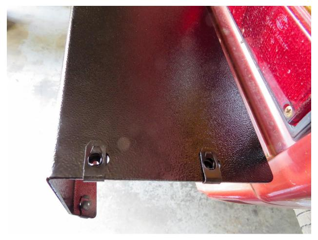
17. Tap three of the smaller j-clips into the three holes in the outer edge of each wing.
