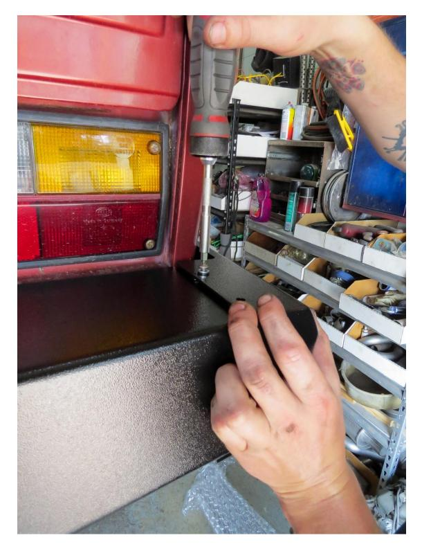
19. Hold the end cap level with the body line of the rear panel and mark the body through the end cap inner mount hole NOTE: While Vans have a hole where the original end cap mounted, this hole only rarely aligns with the mounting hole for the Twin Peaks bumper.
