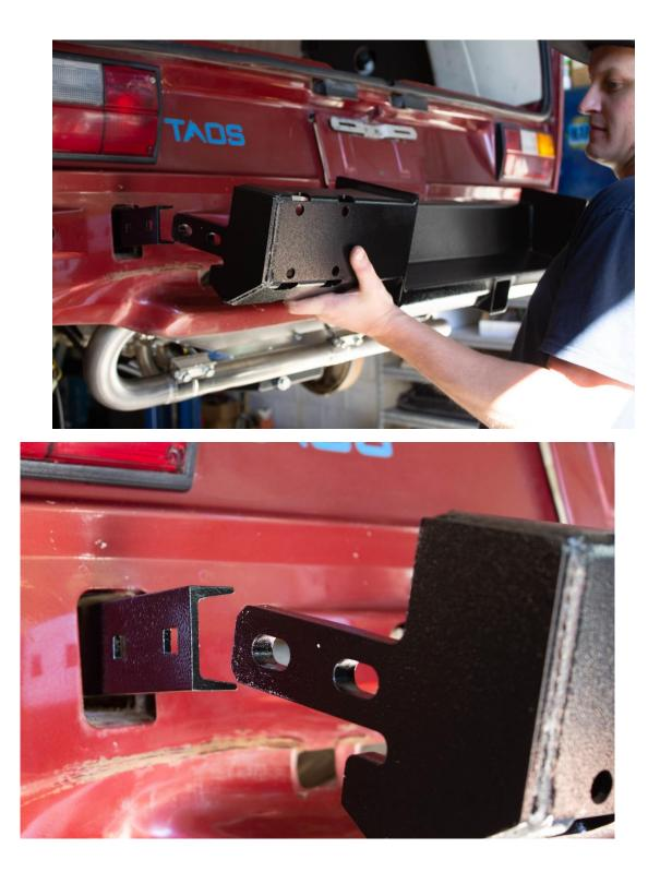
6. Slide a <sup>1</sup>/<sub>2</sub>" carriage bolt through the bracket and center section from the outward side of the bracket. Place a plastic washer and then a metal washer over the bolt followed by a <sup>1</sup>/<sub>2</sub>" nylock nut. Tighten the nuts, leaving them just loose enough to move the center in and out for aligning the bumper. Repeat on the opposite side bracket.
