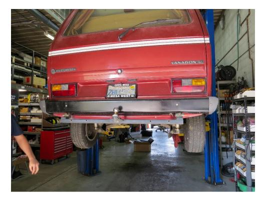
Remove the plastic screw covers on the bumper end cap and remove the Philips head screw from the body.
