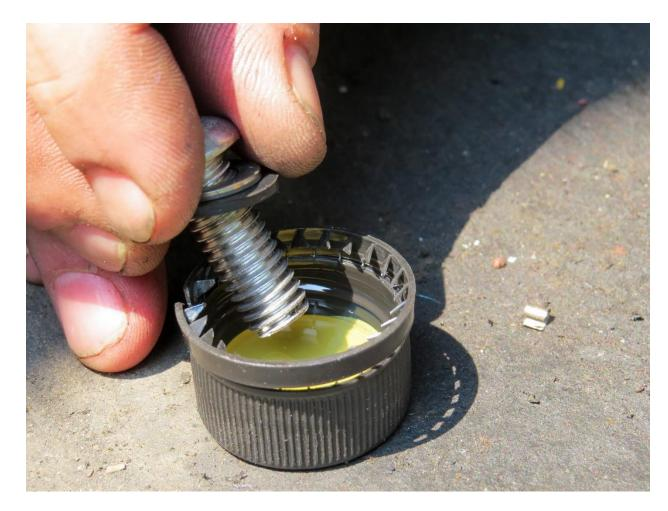
13. Oil the threads of the buttonhead with a small amount of oil.
