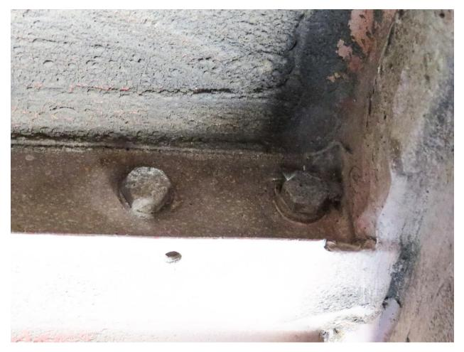
Remove these two bolts on either side and carefully remove the bumper from the Van. Try to avoid nicking the paint when you withdraw the brackets from the Van.
