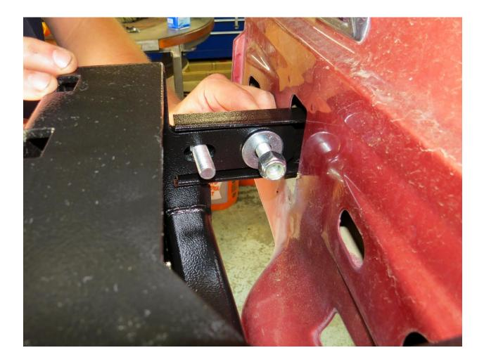
7. Position the center section so that the bottom front edge is about 1/8" from the lower valence of the Van. NOTE: keep in mind that your valence is probably not straight after more than forty years of street use. It is easily bent back away from the bumper if needed.
