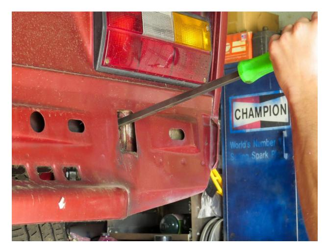
3. Slide the Van Cafe Twin Peaks bumper bracket into the bumper bracket slot as shown with the flat side toward the outside of the Van. Note the square holes are toward the rear of the Van.
