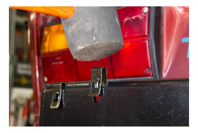
9. Tap all eight j-clips onto both sides of the center section in the orientation shown below.
