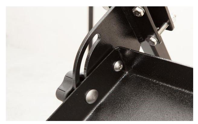
7. Insert a 3/8" carriage bolt through the square hole from the inside of the rim of the tray. Slide a black nylon washer between the shelf and bracket and then push the bolt through the bracket. Add a nylon washer over the threads and then loosely screw on the star-knob. Once again you are protecting the powdercoat with the two nylon washers. Repeat for the opposite side.
