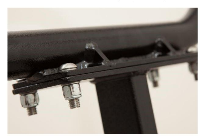
2. Position the shelf mounting bracket under the latch post flange so that the latch post goes through the slot in the bracket and the holes in the three layers of steel align. Insert a 3/8" X 1.25 buttonhead screw and 3/8" washer through each of the holes from the top of the assembly. Thread a 3/8" washer and 3/8" nylock nut onto each and tighten.
