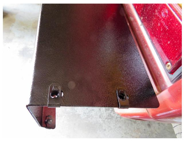
17. Slide the end cap over the wing and, with a buttonhead/metal washer/plastic washer combination, loosely thread the three fasteners through the holes in the end cap and into the j-clips.
