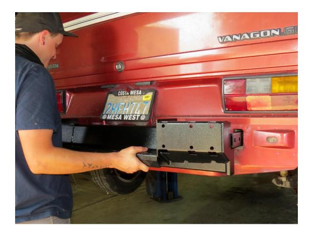
6. Slide a <sup>1</sup>/<sub>2</sub>" carriage bolt through the bracket and center section from the outward side of the bracket. Place a plastic washer and then a metal washer over the bolt followed by a <sup>1</sup>/<sub>2</sub>" nylock nut. Tighten the nuts, leaving them just loose enough to move the center in and out for aligning the bumper. Repeat on the opposite side bracket.
