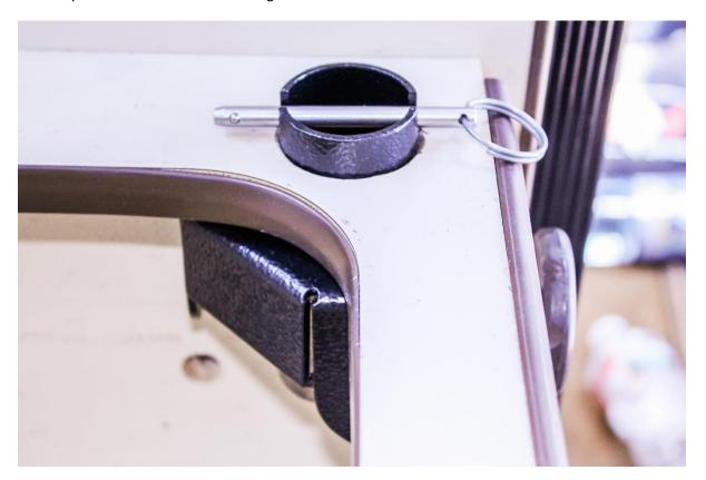
13. To use the table in the bench seat position, simply loosen the factory leg clamp and lift up on the table to pull the pin out of the notch and rotate. The table leg will then rest on the pin and can easily be rotated into position.
