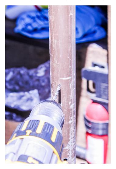
11. Working your way up to a 1/4" drill bit in several small steps is the easiest way to drill the hole to size. The hole needs to be just large enough to insert the lock pin.
