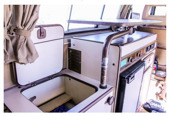
8. Using a permanent marker make a mark on the table leg tube in the center of the notch bracket (on both sides). This will be where you'll drill the table leg tube for the included locking pin.
