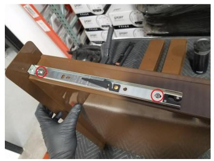
3. Use another (4) #8-32 x 1/4" SS button head screws and nylock nuts to bolt on the outer slide to the RH and LH side pockets as shown.
