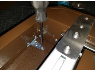
18. To install the magnetic latch plates, pull the inner drawer out and release the drawer slides to remove it from the table and set it aside for now. Ensure the (2) striker pads are still positioned properly on the magnets and install using the small black countersunk screws. With some downward pressure, screw in the screws by hand making sure not to over tighten (Do NOT use a drill!).
