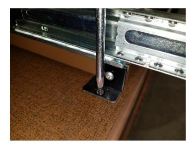
19. Once the magnet latch pads are attached, you may reinstall the inner drawer, again making sure that the slides are properly aligned. Next, pull up on the drawer assembly and lean it back against something so you don't have to hold it up (wall etc...). This will allow for easier access to install the remaining (4) silver screws into the hinges.
