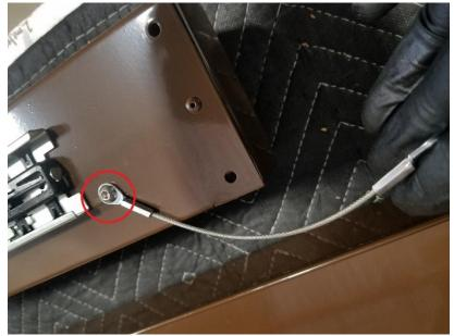
6. Using (4)  $#10-32 \times 5/16$ " SS button head screws and nylock nuts, attach the table hinges to the **back side** of the back cap as pictured.
