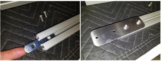
11. With both channels preassembled, you may now flip the table drawer over and gently lay it on the table. Next set each channel onto the bottom of the drawer and align the bolt plates with the holes in the end caps. Attach using (8) #10-32 x 5/16" SS button head screws and nylock nuts as shown. Tip: Hang the end of the drawer off the table slightly to get access to the inside of the end cap. Once the #10 screws have been tightened, you can now tighten the (8) M8 screws as well.
