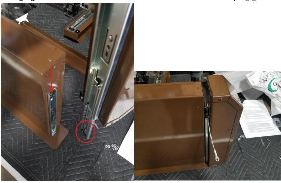
8. You can now attach the back cap to both LH and RH side pockets using (4)  $\pm 10-32 \times 5/16$  SS button head screws and nylock nuts. Doing so on a nice flat surface can aid the assembly.
