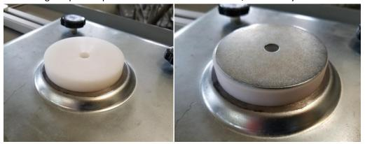
24. Next reinstall the factory wave washer followed by one of the regular washers onto the thumb screw. Then, flip the table leg over and set it onto the slider assembly and install the thumb screw.
