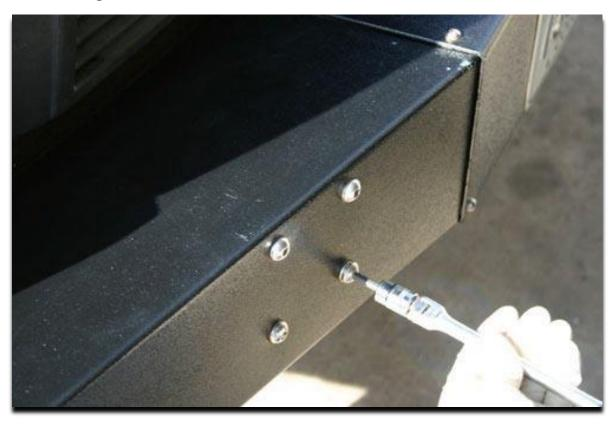
3. You will find new M10 slip-on j-clips in the hardware pack of the Twin Peaks Full Grille Guard. Remove your old j-clips off from your Twin Peaks Front Bumper Mounts and install the new ones in the same positions
