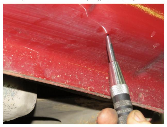
Drill pilot holes with either a 1/8" drill bit or a step drill bit.
