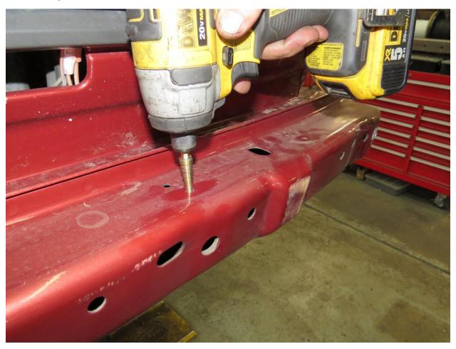
Deburr and use touch up paint on the drilled holes.
