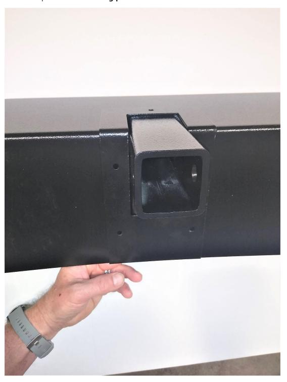
Assemble the included plastic washers, stainless washer and then button head bolt with the plastic toward the powdercoat.
