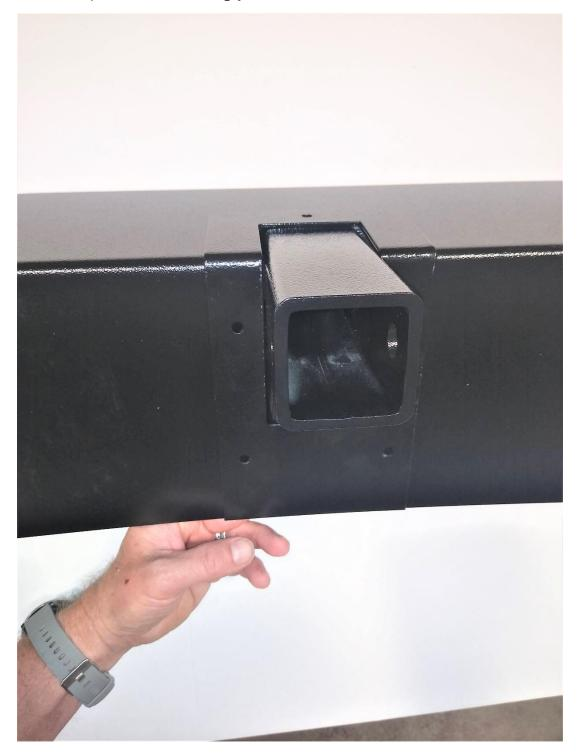
Assemble the included plastic washers, stainless washer and then button head bolt with the plastic toward the powdercoat.
