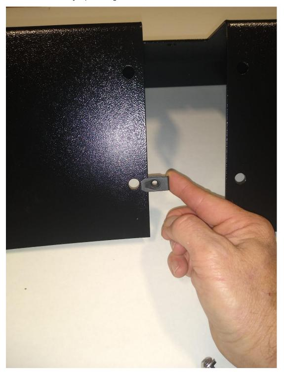
Slide the included 5 j clips through the five holes in the center of the **center cover**.
