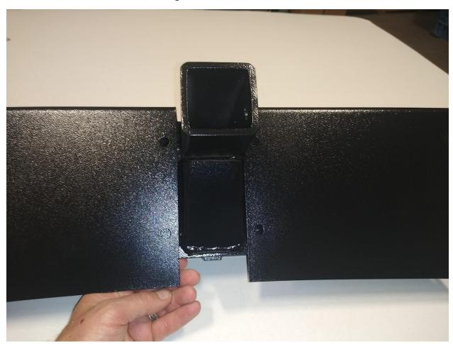
Reinstall **center cover** over the wings and **receiver**.
