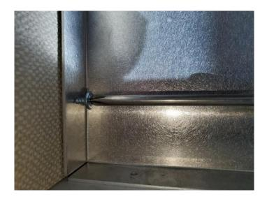
**Step 4:** Measure the rear again to make sure it's still 4" to the tray edge and install another screw in the rear hole to secure it in place. You can also now install the passenger side center screw as well.
