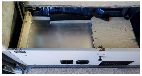
**Note:** This Tray includes an access panel that allows you to still be able to turn on or off the coolant control valve for the factory rear heater (not shown on these instructions). To remove the panel, simply unscrew the thumbscrew and remove the panel. Installation is the opposite of removal.
