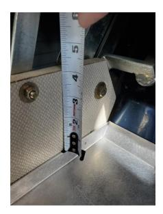
**Step 3:** With the tray at the correct height and pulled tight to the front panel and passenger side of the seat base, install one of the provided truss-head screws in the front hole by using a #2 Philips head screwdriver (Do not use a drill!).
