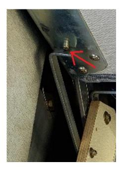
**Step 2:** Next, drop in the tray and measure 4" down from the passenger side edge of the seat base to the top edge of the tray. Do this on the front and back to ensure it's at the same height.
