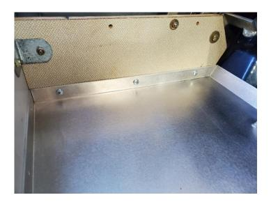
**Step 5:** Now move to the driver's side of the tray, and simply flush it up to the top face of the inner wood panel of the heater cover as shown below. Install a screw to secure it in place and repeat the process in the rear followed by the middle screw.
