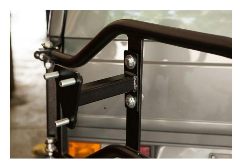
Place a 1/2 Flat Washer and a 1/2 Nylock Nut onto each of the Hex Head Bolts.
