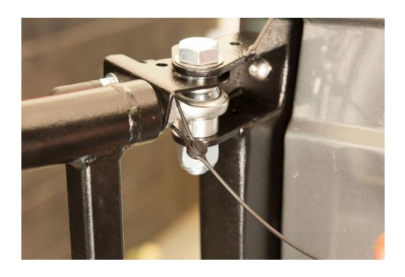
The loop on the end of the **Nylon Lanyard** is to be threaded onto the key ring of the **SS Quick Release**
