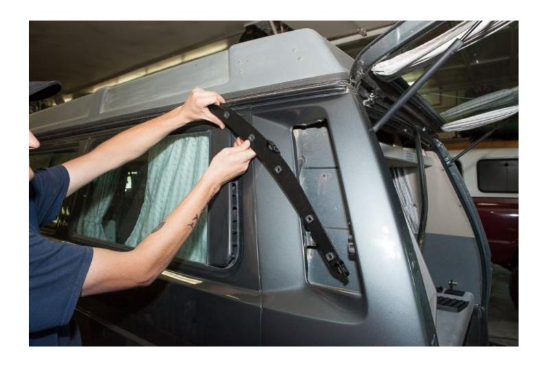
While the **Support Backing Plate** is being held in place, thread the two **3/8x16x4" LG All Thread Rods** from **Hardware Package A** into the rear of the van insuring that they grab and thread into the **Cage Nuts** on the **Support Backing Plate**. These **All Thread Rods** are used as an installation guide and will help keep the **Support Backing Plate** in its proper location for the duration of the installation.
