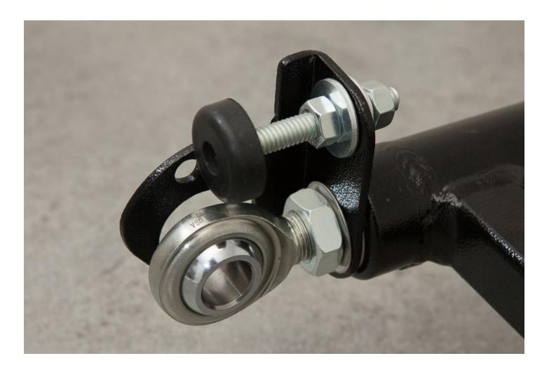
Assemble the lower contact point of the **Swing Arm** by using hardware from **Hardware Package B.** Take one of the **5/8x18 Heim Joints** and thread a **5/8x18 Jam Nut** onto it followed by a **5/8 Flat Washer.** Now thread this entire assembly into the **Swing Arm**.
