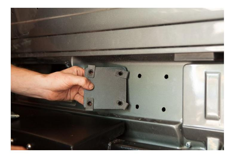
With one hand place the **Striker Backing Plate** through the tail light opening and up against the backside of the van where you drill the mounting holes. The **U-Nut Slip-Ons** should line up with the four holes you've drilled.
