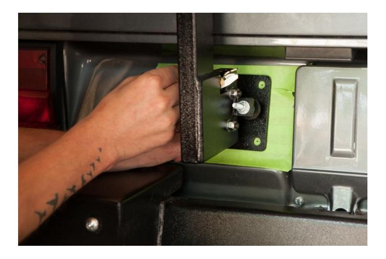
Once all four holes have had their center points located with a **Sharpie**, swing the **Swing Arm** out of the way. Use a **Center Punch** in order to create an indention at all of the marks you've made. These indentions will help keep your drill bit in place and not "walk away" during the drilling process.
