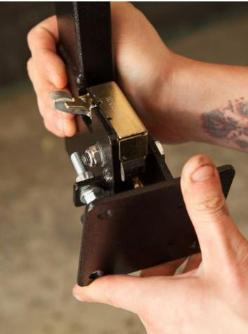
Swing the **Swing Arm** into the closed position so that the back of the **Striker Plate** butts up against the van.
