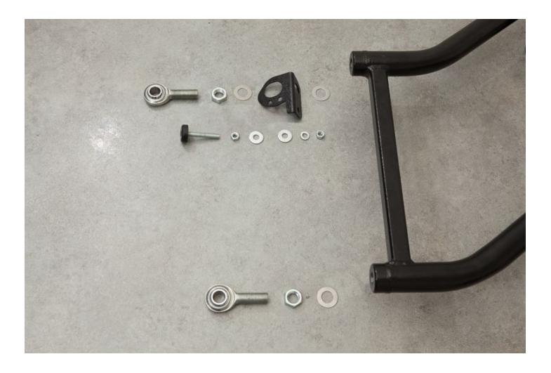
Assemble the **Bump Stop Plate** by using the **5/16x18x2" LG Foot Adjuster**, **5/16x18 Nut (x 2)**, **1/4 Washer (x 2)** and a **5/16 Lock Washer (x 1)** from **Hardware Package B.** Leave the finished assembly loose as it will be fine tuned and locked into place later in the installation.
