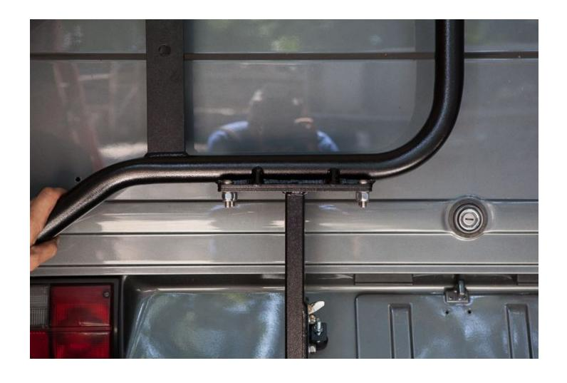
Now that the location is correct. Place the lower **Heim Joint** into the lower slot of the **Support Plate**. Add one **7/16 Aluminum Heim Spacer** from **Hardware Package B** above and below the **Heim Joint**.
