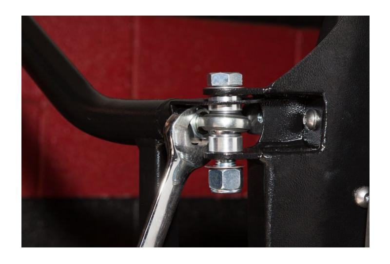
Use a 15/16" Wrench in order to fully tighten down the Jam Nut on the lower Heim Joint.
