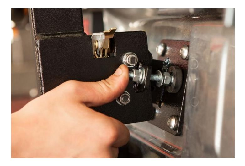
Use two 13mm Wrenches in order to fully tighten the Jam Nuts on the Foot Adjuster.
