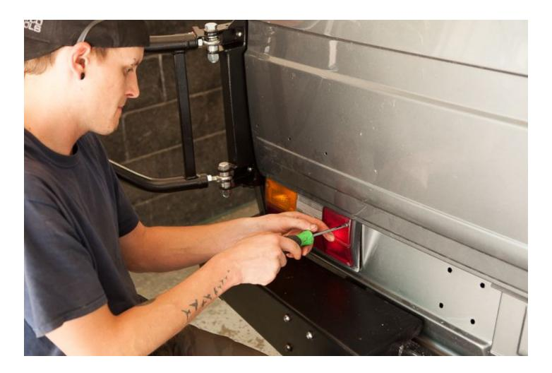
Orientate the **Striker Backing Plate** as shown with the flat sides of the **U-Nut Slip-Ons** facing towards the rear of the van. This is how it will need to sit behind the van body.
