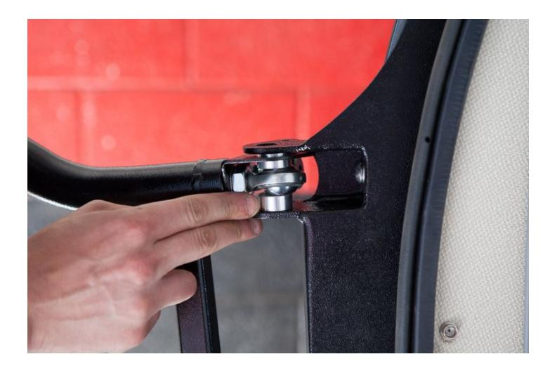
Place a **5/8 Flat Washer** on top of the **Support Plate** and then insert a **5/8x11x3" LG Hex Head Bolt** from **Hardware Package B** through the assembly.
