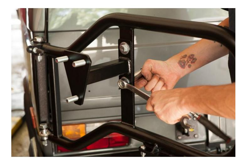
Place your spare tire onto the three studs on the **Tire Mount Stand Off.** Use a **19mm Socket** and **Ratchet** in order to tighten the three **14x1.5 Lug Nuts** into place.
