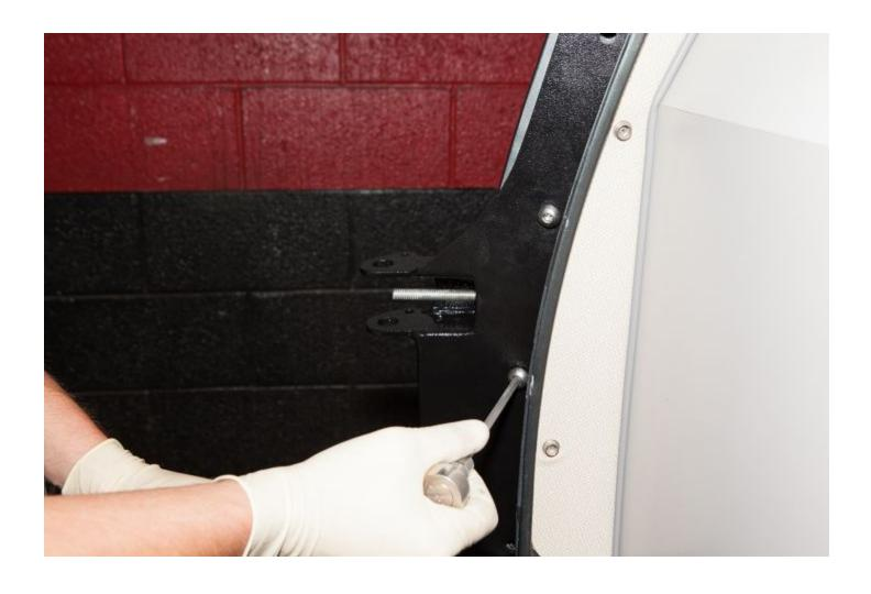
Remove both **All Thread Rods** that were in place as guides. Use a **5.5mm Hex Bit Socket** and a **Ratchet** in order screw the two **SS Button Head Screws** into the front side of the **Support Bracket**.
