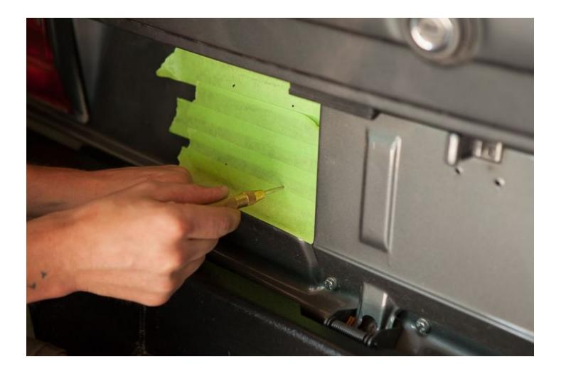
Use a **Drill** and a **1/8" Drill Bit** with a **Stop Collar** in order to drill your pilot holes. Set the location of the **Stop Collar** about a half inch from the tip of the **1/8" Drill Bit**. The **Stop Collar** will allow you to drill through your van's body without accidentally pushing all the way through and possibly damaging something on the other side.
