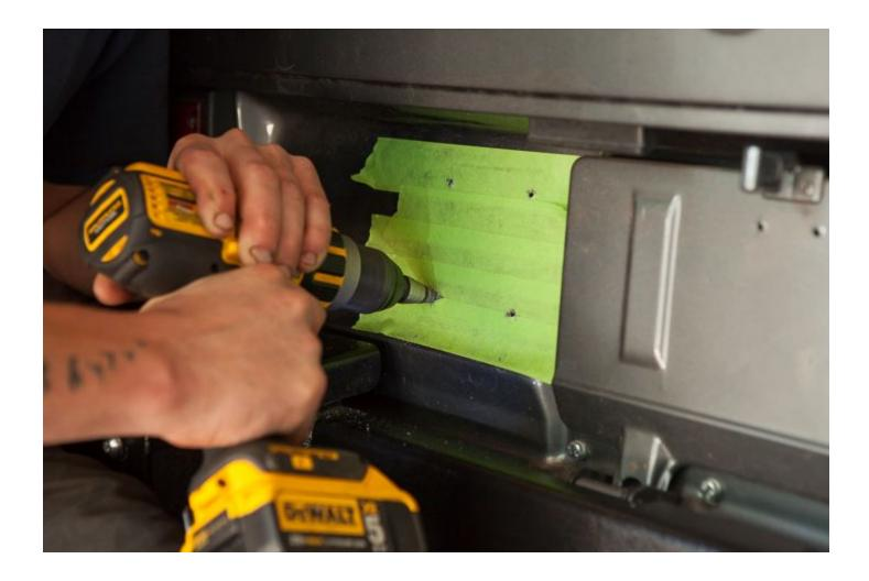
Use a **Deburring Tool** on your **Drill** in order to remove and metal flashing on the seven 7/16" diameter holes you've just drilled. This will clean up the edges nicely which should make them smooth to the touch once completed.
