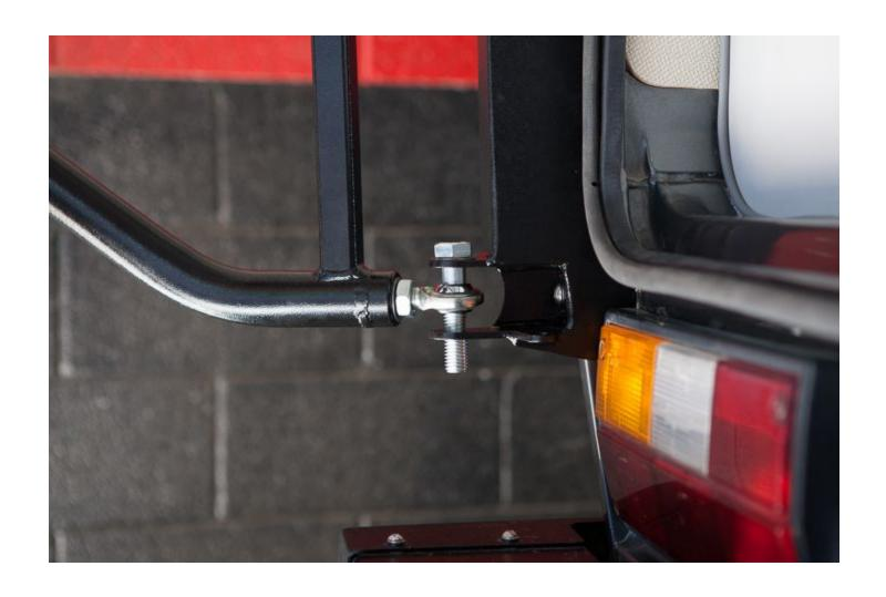
Close the van's rear hatch door. Swing the **Swing Arm** to a simulated closed position. Notice the horizontal member of the **Swing Arm** is not parallel with the lines in the van itself. We need to adjust
