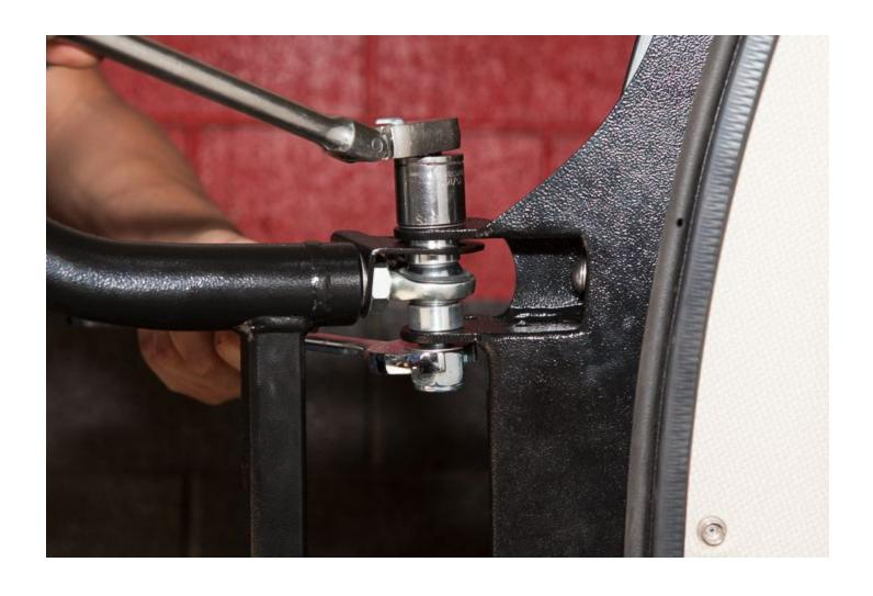
Use a **15/16" Wrench** and a **15/16" Socket** on a **Rachet** in order to fully tighten down the **Hex Head Bolt** and **Nylock Nut** on the lower **Heim Joint**.
