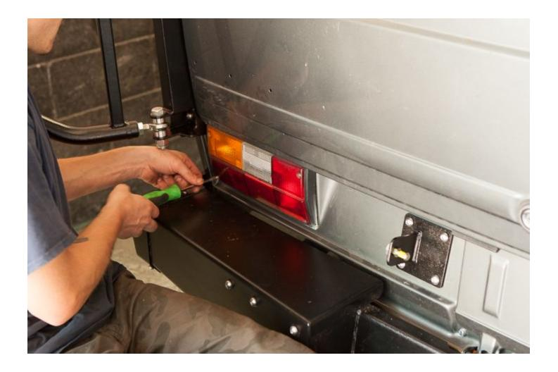
Swing the **Swing Arm** closed and let the **Latch Lock** connect to the **Striker Pin.**
