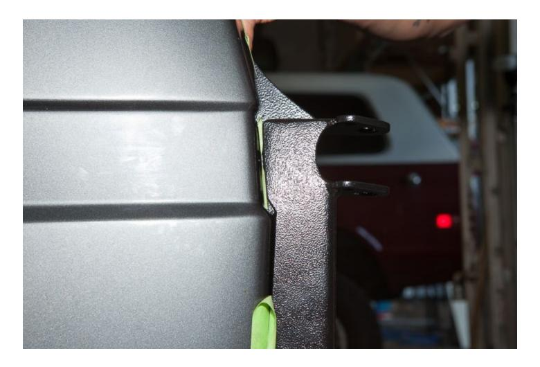
The second point of reference is a small bump that resides in the pillar. We have a small area of the **Main Support Bracket** removed in order to accept that small bump.
