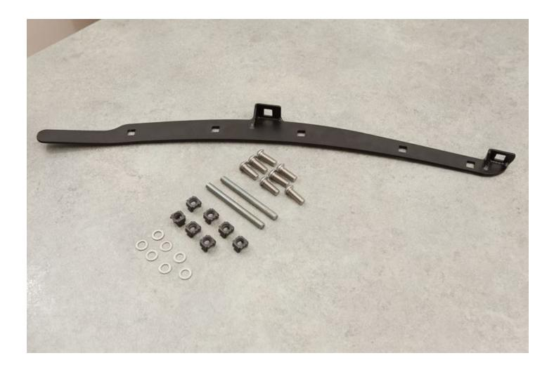
The seven included **3/8x16 Cage Nuts** are to be inserted into the rectangular slots in the **Support Backing Plate.** Place one end of the **Cage Nut** into the slot, then squeeze the spring clip and apply downward pressure making the **Cage Nut** seat completely.
