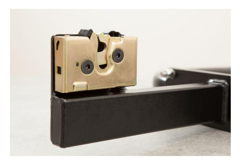
Place a **5/16 Washer** and a **8x1.25 Nylock Nut** from **Hardware Package D** onto each of the **Allen Head Screws.** Use a **Drill** with a **5mm Hex Bit Socket** and a **13mm Wrench** in order to securely fasten the **Locking Latch** to the **Latch Post**.
