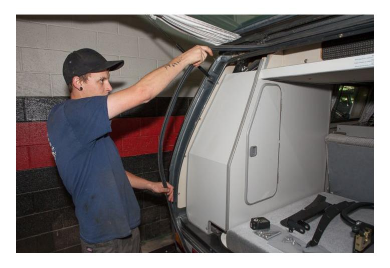
Place **Masking Tape** on the van's body as shown. This layer of **Masking Tape** will help protect your van's paint from the **Main Support Bracket** while you test fit it in order to locate the holes to be drilled.
