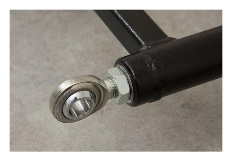
If you have difficulty threading the **Heim Joints** into the Swing Arm you can use on the of the **5/8x11x3" LG Hex Head Bolts** located in **Hardware Pack B** in order to help get more leverage on the **Heim Joint** while threading it into place.
