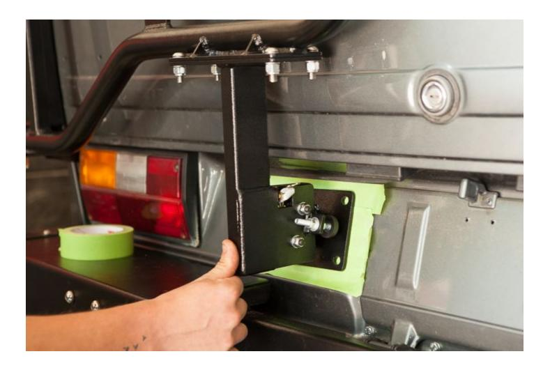
Use a **Sharpie** in order to locate the center point of the four mounting holes in the **Striker Plate.**
