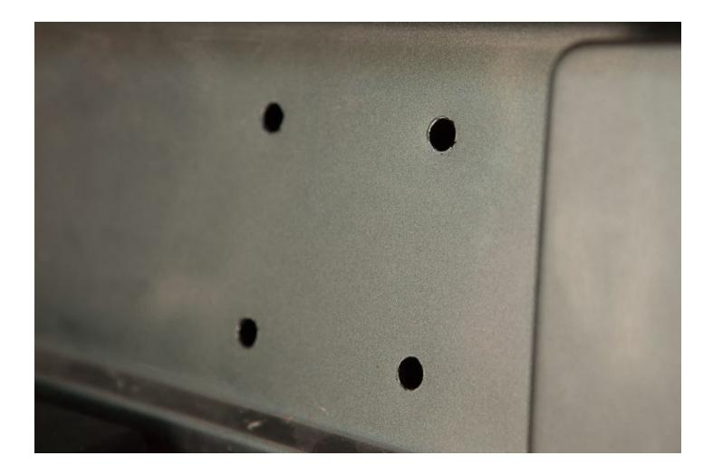
Use a **Phillips Head Screwdriver** in order to remove the four mounting screws holding the driver's side tail light in place. Remove and unplug the tail light.
