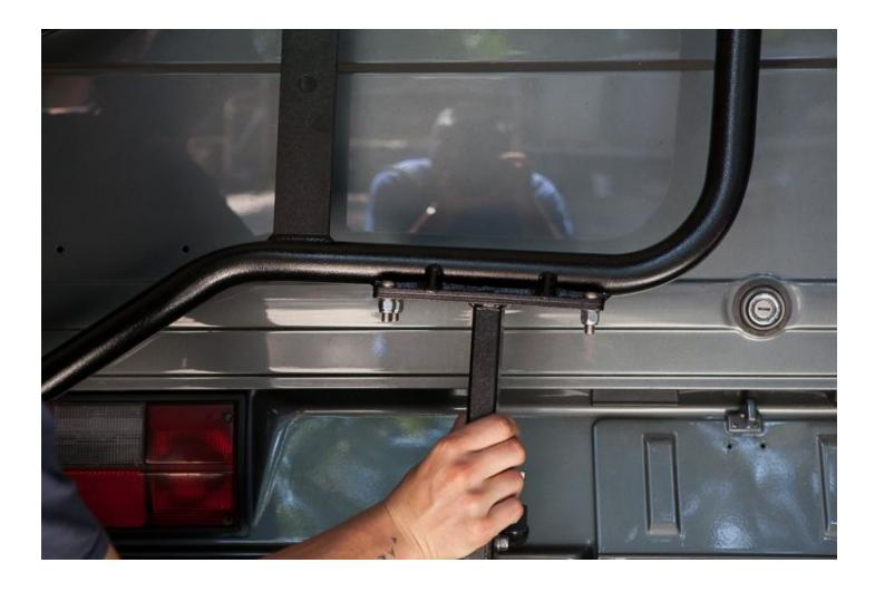
This is the corrected position of the **Swing Arm.** We want the **Swing Arm** level with the horizontal lines of the van.
