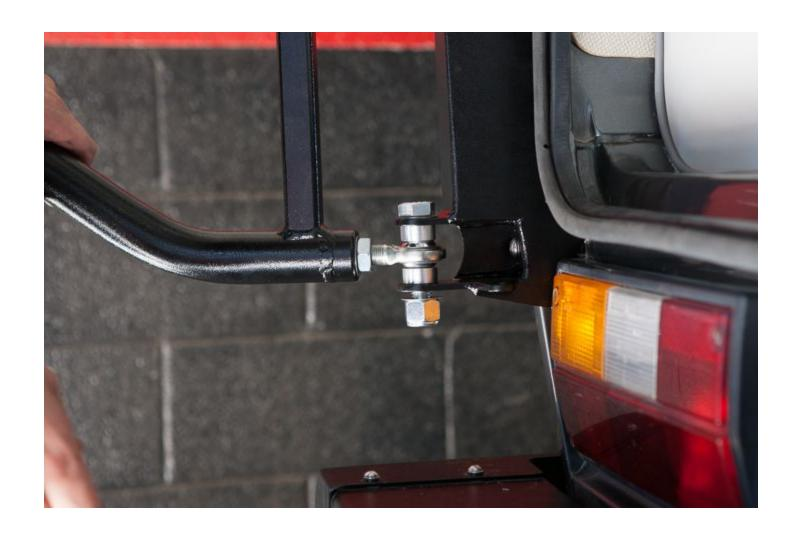
Use a 15/16" Wrench in order to fully tighten down the Jam Nut on the upper Heim Joint.
