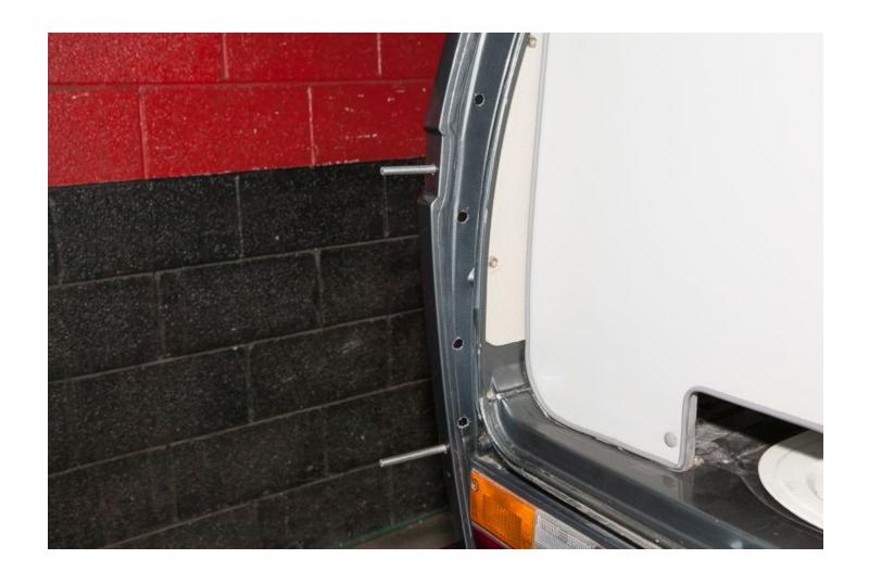
Slide the **Support Plate** onto the **All Thread Rods** that you've threaded into the **Support Backing Plate**.
