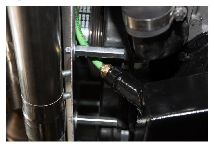
3. Slide the included p-clamp over the top of the dipstick in such a way that the flat part of the clamp rests against the heat shield. Insert a bolt from the engine side of the p-clamp and through the bracket and heat shield. Loosely install a washer and nut on the rear side of the heat shield. The dipstick tube will be positioned in between the two bracket mounting bolts. See photo below for reference.
