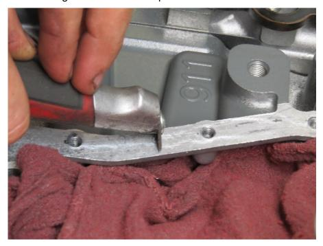
...and finish removing the factory gasket sealant with a 3M pad. The cleaner your surface, the better chance of a leak-free seal: take your time and be thorough!
