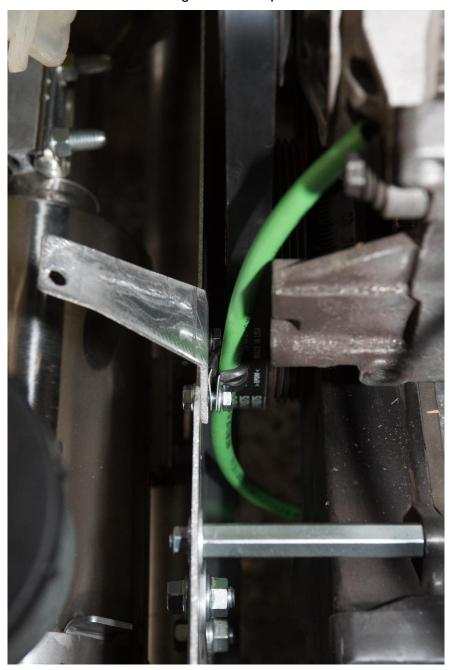
4. Slide the black plastic routing clamp over the dipstick tube so that the bolt hole on the clamp lines up with the bolt hole on the righthand side of the bracket. Insert a bolt through the clamp and bracket and loosely install a nut onto the exposed threads.
