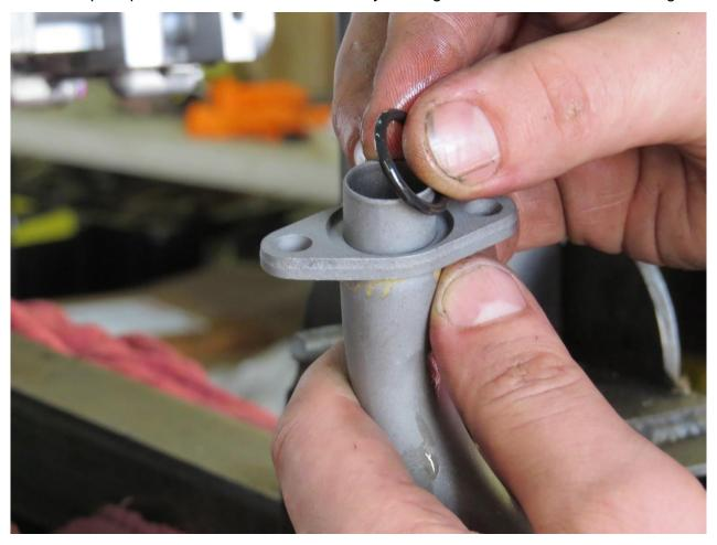
9. Use the two original bolts to bolt the RMW pickup tube to the block making sure the o-ring seats into the block evenly. Make sure the tube is oriented as shown in the photo. Torque these bolts to 10nm.
