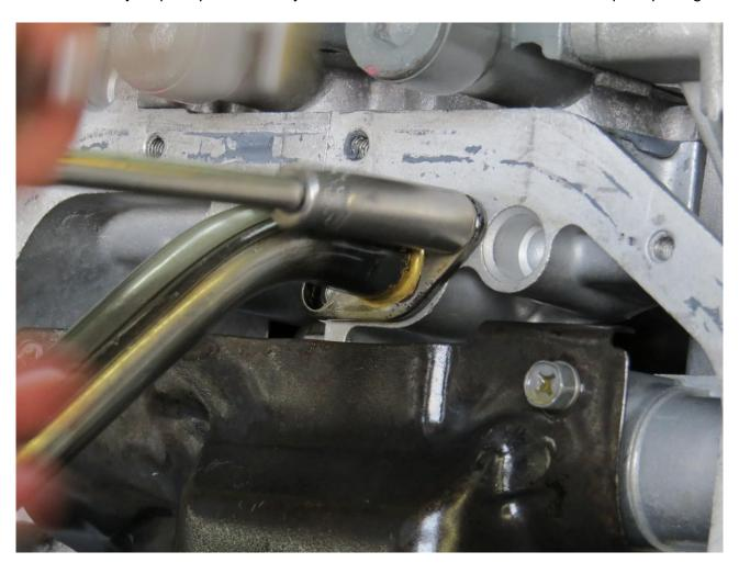
5. Then remove the third bolt at the oil pickup bracket.
