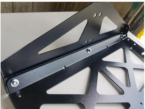
3. (Important) If your storage box measures 24", you may attach the two side gusset plates using the included (8) ¼" Carriage bolts, (8) ¼" Washers, and (8) ¼" nylock nuts as shown. If your storage box is wider than 24" however, install just the upper 4 bolts as shown in the 3<sup>rd</sup> picture below:
