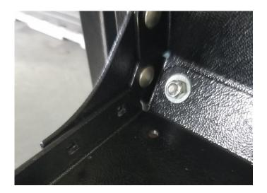
4. Next, install the mount to your half-swing using the included (2) ½" Bolts (4) ½" washers (2) ½" nylock nuts. The mount has two sets of holes. In this case, we are using the RH set of holes to mount the bracket on the Driver's side of the Van. (Important!) Before tightening the bolts, use a bubble level to ensure the mount is level with the swing in the closed position.
