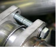
You will use the M8 x 45mm hex bolts with two of the conical Belleville washers stacked under each bolt head, and the flanged copper nuts with no washers to pull the captive flanges together, as shown above right. Slip the joints together, thread up the bolts, cone washers, and nuts, and tighten the nuts until the joints are brought together snug, but don't final tighten the fasteners yet.
