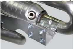
Another band clamp should be slipped in the opposite direction onto the 2" collector pipe end of the secondary. The clamp's bolts should be to the rear and the nuts downward so they will be easier to access. Next slide the J-pipe to the left enough that you can slip the longer leg of the J-pipe and the end of the secondary pair together.
