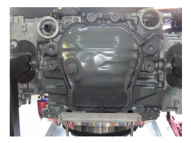
3. Once you have the bolts removed, you may have to use a plastic scraper to wedge the pan apart from the engine block. Do NOT use anything metal here as you will mar the aluminum of the block's sealing surface.
