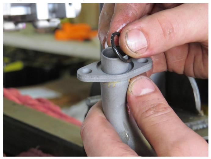
9. Use the two original bolts to bolt the RMW pickup tube to the block making sure the o-ring seats into the block evenly. Make sure the tube is oriented as shown in the photo. Torque these bolts to 10nm.
