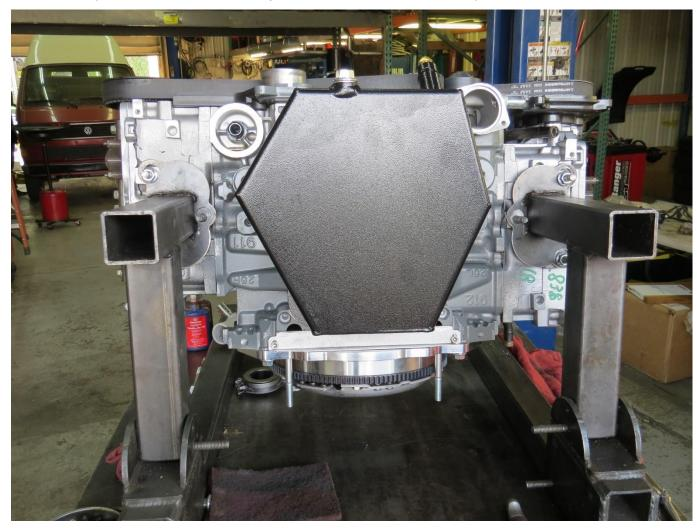
13. You'll be installing the dipstick tube after the exhaust heat shield. We recommend temporarily placing tape over the dipstick tube fitting on the pan to prevent debris intrusion.
