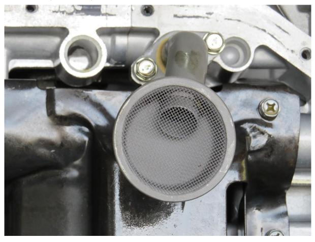
10. Once the tube is bolted in, test fit the oil pan onto the motor. All good? If so then it's time to add a little sealant and bolt in the pan. Here at the shop we use Permatex "The Right Stuff" gasket maker and apply a small 1/8" bead around the engine to oil pan mating surface. Make sure you circle the bolt holes to ensure proper sealing. DO NOT use too much sealant – more is not better in this instance!
