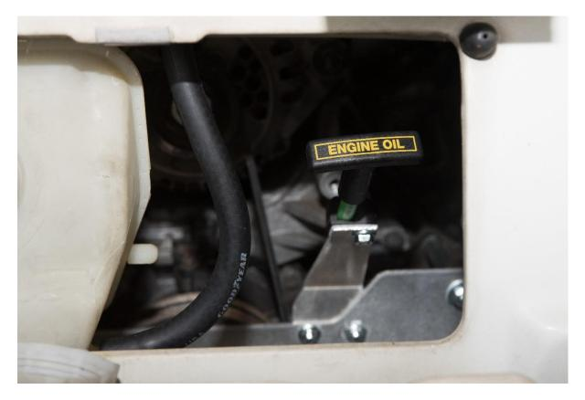
Prime and install Subaru filter and fill with approximately 4.5 quarts of 5W/30 motor oil for the 2.5 liter and 10W/30 for the 2.2 liter. Refer to Subaru specifications pertaining to your specific engine for oil type, weight and service intervals.
