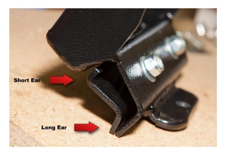
Use the contents of **Hardware Package A** in order to loosely bolt up the **Rain Gutter Keeper Plate** to the **Main Support Bracket**. The **Rain Gutter Keeper Plate** has two square holes in it which allow for the included **Carriage Bolts** to mount through in order to keep them from turning as you tighten the **Nylock Nuts** later in this installation. Loosely bolt up both sets of brackets.
