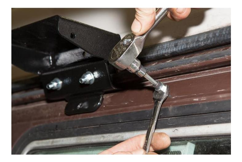
Once the **Rivet Nut** is set, remove the hardware you've used to set it in place. Your **Rivet Nut** should be nice and secure into the body of the van. This additional mounting location will help secure the **Road Shower Support Brackets** in place and help carry the load of a filled Road Shower.
