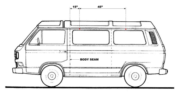
We'll install the bracket closest to the front of the van first. Slip the loosely assembled **Main Support Bracket** and **Rain Gutter Keeper Plate** onto the rain gutter of the van. Locate the center of the hole in the foot of the **Main Support Bracket** 15" from the vertical body seam that's right behind the driver's front door like the previous graphic shows.
