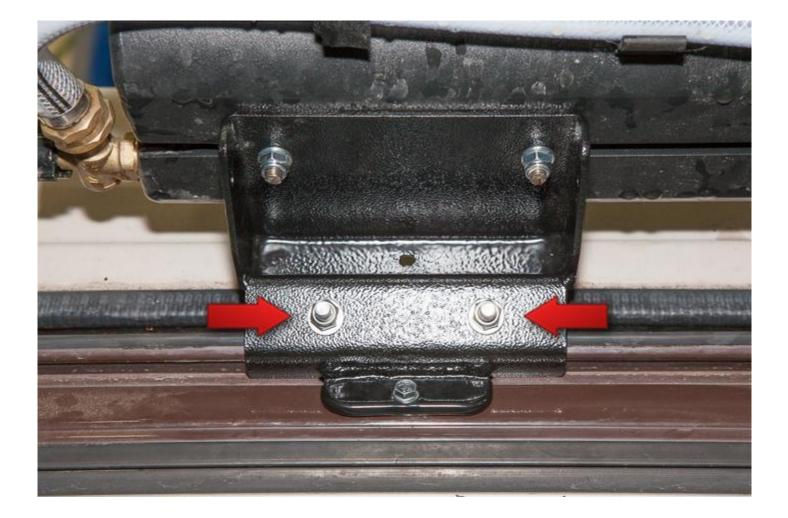
Place the Security Plate in place making sure the tabs on the Security Plate are inserted into the holes on the Main Support Bracket.
