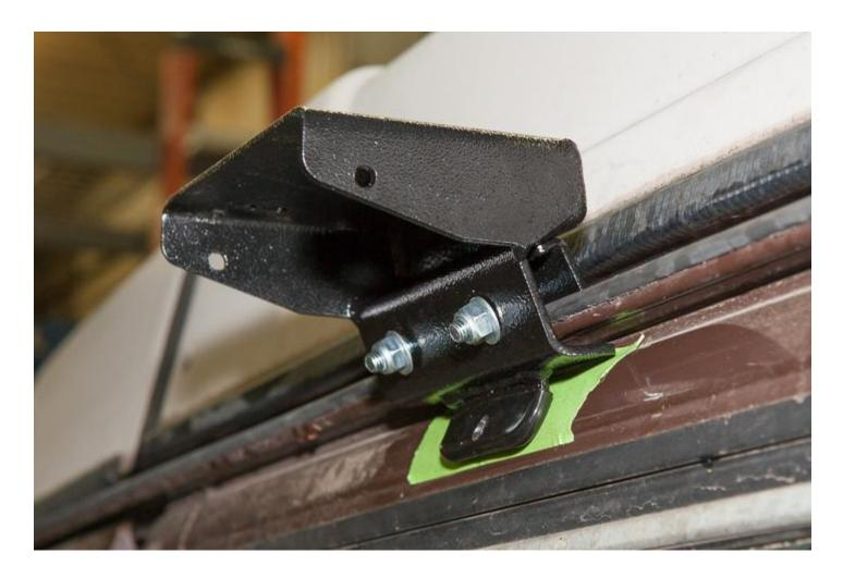
Use a <sup>1</sup>/<sub>2</sub>" Socket, 6" Socket Extension and Ratchet in order to tighten down the Nylock Nuts with Flat Washers. This will help snug the bracket up to the rain gutter.
