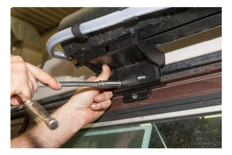
We recommend installing a 5/16" Locking Knob onto the other exposed **Carriage Bolt** making your installation completely secure. This locking knob will keep thieves from being able to access any of the mounting hardware which makes your investment completely safe from theft.
