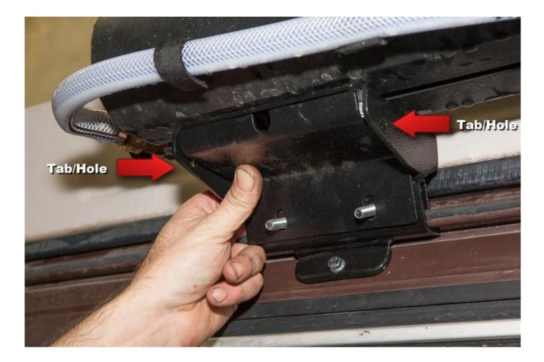
Use a <sup>1</sup>/<sub>2</sub>" Socket, 6" Socket Extension and Ratchet in order to reinstall the Nylock Nut and Flat Washer on one of the exposed Carriage Bolts.
