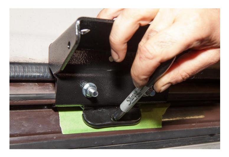
The reason we mark the hole **AFTER** tightening down the bracket assembly is to be certain that the **Rivet Nut** that we're about to install lines up correctly with the hole in the lower bracket once the bracket is tightly secured.
