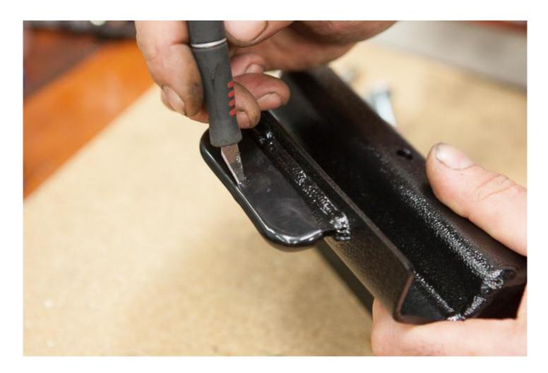
The finished product should look like this. The rubber cover was cut from both sides exposing the mounting hole in the **Main Support Bracket** foot. This will allow a mounting bolt to be used without the interference of the rubber cover.
