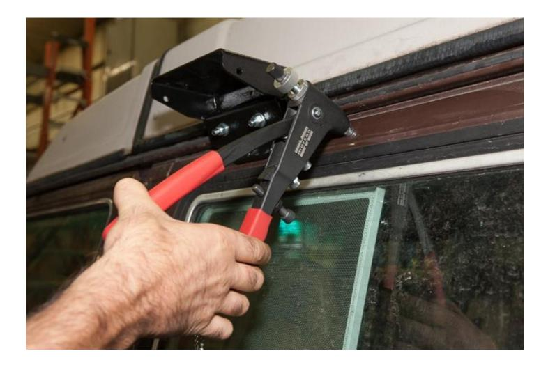
Slide the Road Shower Support Bracket back into place. Use a ½" Socket, 6" Socket Extension and Ratchet in order to tighten the Nylock Nuts back down.
