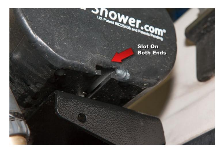
The square shoulders of the **Carriage Bolts** will drop right into the slot on the bottom keeping the **Carriage Bolts** from rotating as you tighten them down.
