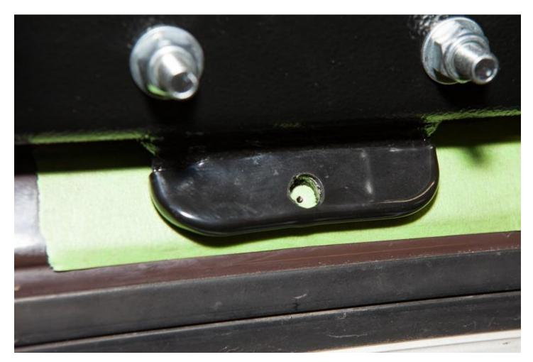
Use a <sup>1</sup>/<sub>2</sub>" **Socket**, **6**" **Socket Extension** and **Ratchet** in order to loosen the **Nylock Nuts**. Once the **Nylock Nuts** are loosened slide the assembly down the rain gutter exposing the mark on the **Masking Tape** you just made.
