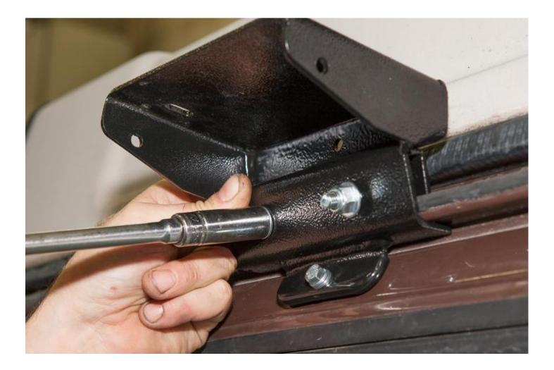
Use a 10mm Socket, 6" Socket Extension and Ratchet in order to tighten the Bolt, Lock Washer and Flat Washer found in Hardware Package B into the Rivet Nut.
