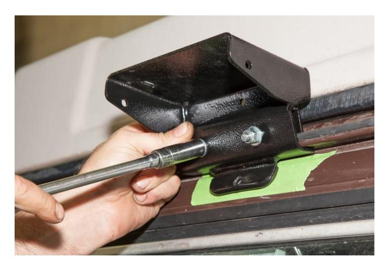
Now that the **Main Support Bracket** and **Rain Gutter Keeper Plate** are firmly in place we can locate the center point of the hole that we need to drill into the side of the van. Use a **Sharpie** to mark the center of the hole in the **Main Support Bracket Foot**.
