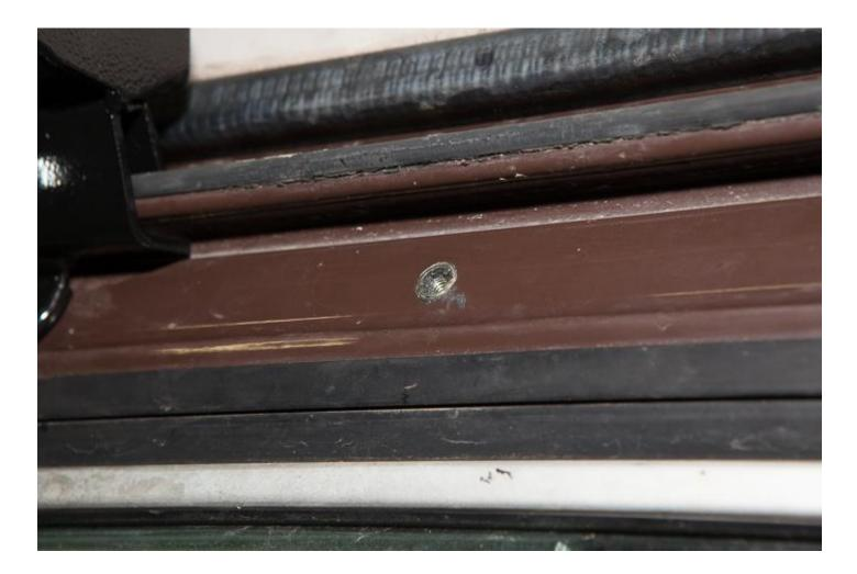
In **Hardware Package D** there are the pieces required in order to properly seat the **Rivet Nut**. The photo below shows the correct orientation of the **Allen Bolt**, **Flat Washer**, **Hex Sleeve** and **Lock Washer** in relationship to the **Rivet Nut** that you just placed into the hole drilled in your van.
