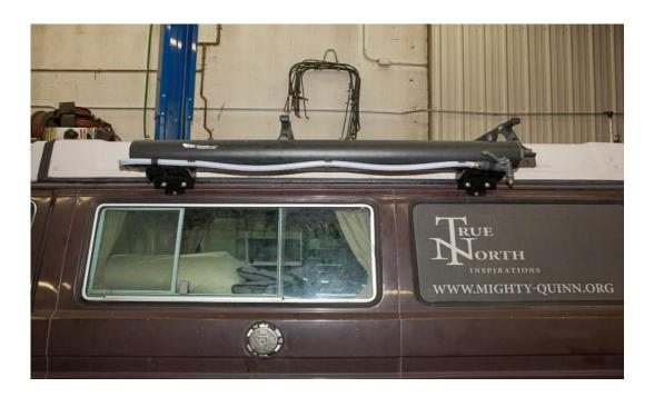
Now you can easily fill, pressurize and/or use your Road Shower easily even with the Top Popped in camping mode. The lower mounting configuration makes the Road Shower more usable in our opinion as well as it helps keep the 45lb setup off of the roof which means lifting the Pop Top is easier.
