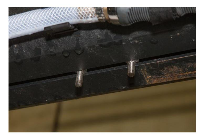
Lift one end of the Road Shower up and slide **two 5/16x.75**" **Carriage Bolts** down so that they feed through the mounting holes on the top base plate of the **Road Shower Support Bracket**. Do this at both bracket locations so that all four **Carriage Bolts** feed through the **Road Shower Support Brackets**.
