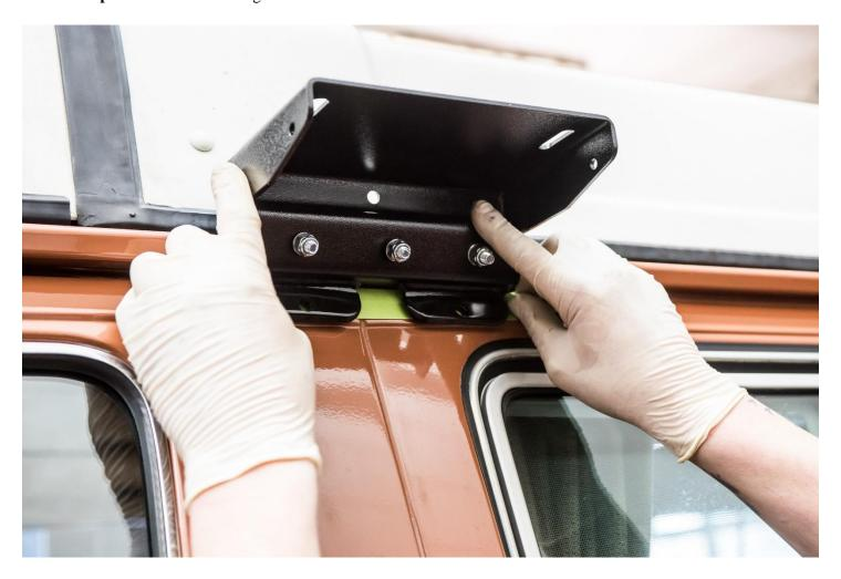
Use a ½" Socket, 6" Socket Extension and Ratchet in order to tighten down the Nylock Nuts with Flat Washers. This will help snug the bracket up to the rain gutter.
