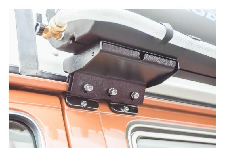
One recommended option is to use a 5/16" Locking Knob onto one of the exposed **Carriage Bolts** to make your installation secure. This locking knob will keep thieves from being able to access any of the mounting hardware and makes your investment completely safe from theft. These can be obtained from most vendors that sell sport racks.
