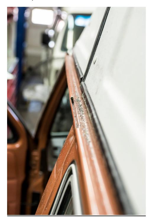
Now we will be making small cutouts in the gutter to accommodate the mounting bolts. Hold the **Rain Gutter Keeper Plate** in the position in which it will be mounted and note that the outer edge of the gutter interferes with the bolt holes. This is the section of gutter that requires clearancing.
