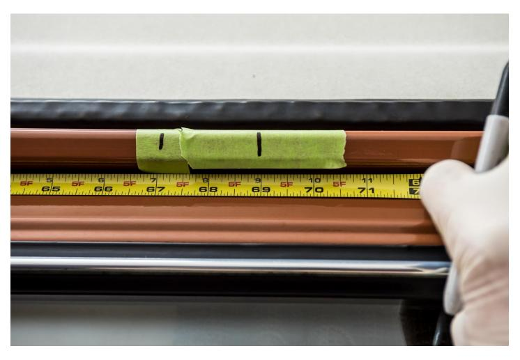
We'll install the bracket closest to the front of the van first. Slip the loosely assembled **Main Support Bracket** and **Rain Gutter Keeper Plate** onto the rain gutter of the van.
