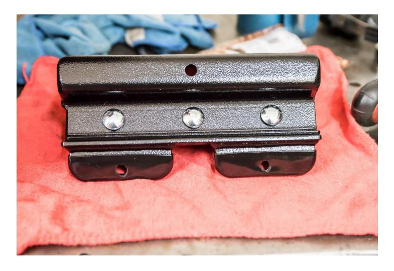
Take the **Rain Gutter Keeper Plate** and orientate it with the **Main Support Bracket** as shown. It is key that the short ear of the **Rain Gutter Keeper Plate** is towards the flat platform of the **Main Support Bracket** and the long ear is towards the foot with the rubber cover.
