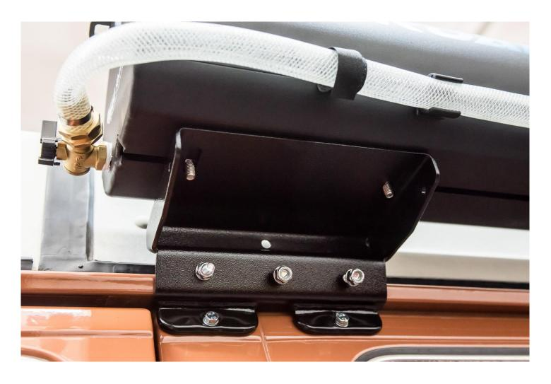
Center the Road Shower cylinder onto the two **Road Shower Support Brackets**. Once confident with the location, use a **1/2" Socket**, **6" Socket Extension** and **Ratchet** in order to tighten the nylock nuts/flat washers found in your original Road Shower Kit.
