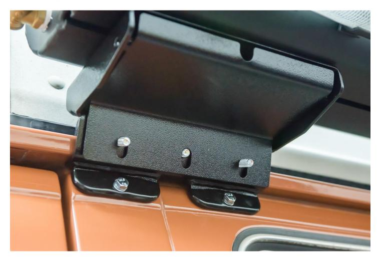
Attach the flat washers and nylock nuts and use a ½" Socket, 6" Socket Extension and Ratchet to tighten.
