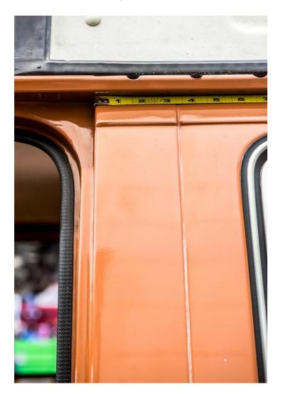
**Front Mount:** For the 4L, place a 12" long strip of **Masking Tape** horizontally from the "B" pillar toward the rear of the Van in to help protect the paint when drilling into the van. For the Road Shower 4 and 4S, place a 12" strip of masking tape centered at about 15" from the "B" pillar.
