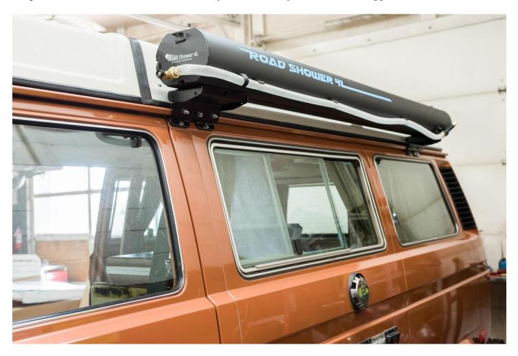
Now you can easily fill, pressurize and/or use your Road Shower easily even with the Top Popped in camping mode. The lower mounting configuration makes the Road Shower more usable in our opinion as well as it helps keep the 45lb setup off of the roof which means lifting the Pop Top is easier.
