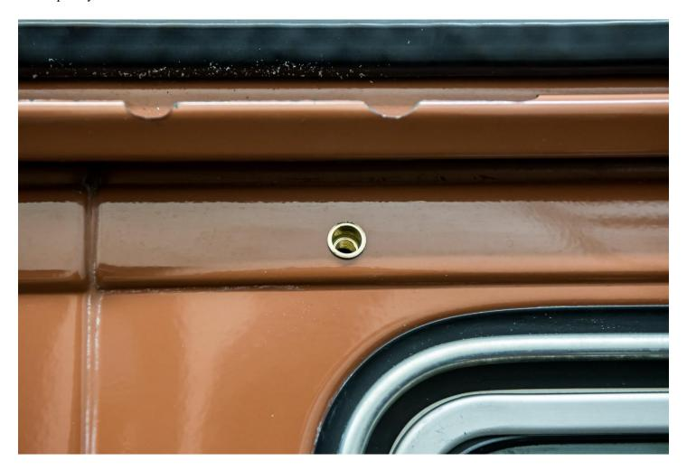
Center the Road Shower bracket feet over the attachment points you just mad in the body of your Van. Use a **10mm Socket, 6" Socket Extension** and **Ratchet** in order to tighten the nylock nuts. The insert the **Bolt, Lock Washer** and **Flat Washer** found in **Hardware Package B** into the **Rivet Nut**. Tighten into place.
