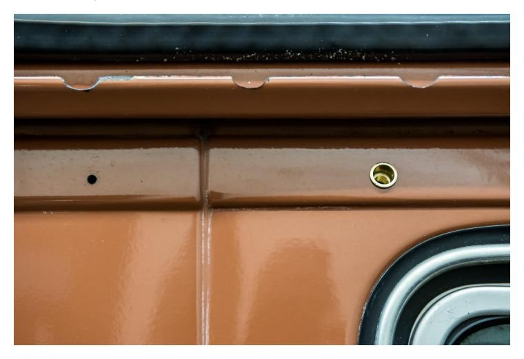
Thread the **Allen Bolt** into the **Rivet Nut** and use a **Ratchet** and **5mm Hex Bit Socket** to tighten the **Allen Bolt** while using a **11mm Wrench** to hold the **Hex Sleeve** in place. As you tighten the **Allen Head Bolt**, a portion of the **Rivet Nut** inside of the van will collapse on itself making the **Rivet Nut** lock in place. Continue to tighten the **Rivet Nut** until you feel it collapse and lock on itself.
