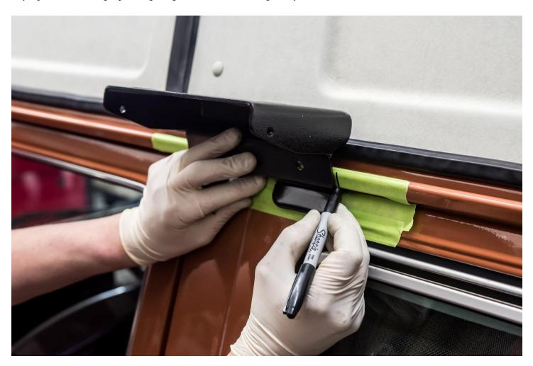
Carefully begin to file the gutter between your two marks. At this point you are just taking off the top inside lip of the gutter.
