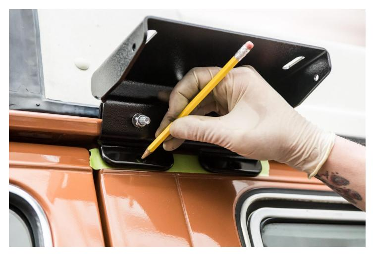
The reason we mark the hole **AFTER** tightening down the bracket assembly is to be certain that the **Rivet Nut** that we're about to install lines up correctly with the hole in the lower bracket once the bracket is tightly secured. Once marked, loosen the nylock nuts and slide the assembly down the gutter out of the way.
