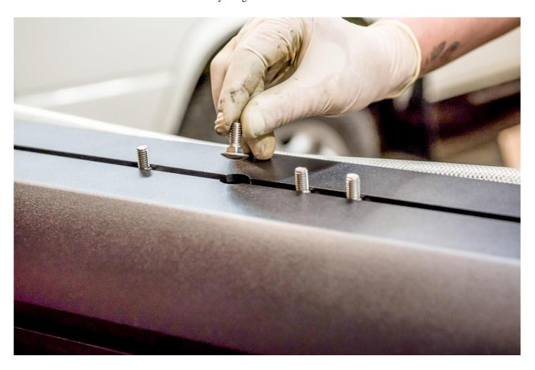
Lift one end of the Road Shower up and slide **two 5/16x.75**" **Carriage Bolts** down so that they feed through the mounting holes on the top base plate of the **Road Shower Support Bracket**. Do this at both bracket locations so that all four **Carriage Bolts** feed through the **Road Shower Support Brackets**. A helper can be valuable here.
