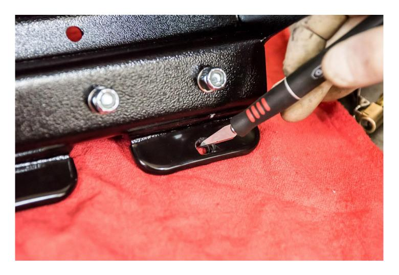
The finished product should look like this. The rubber cover was cut from both sides exposing the mounting holes in the **Main Support Bracket** feet. This will allow a mounting bolt to be used without the interference of the rubber cover.
