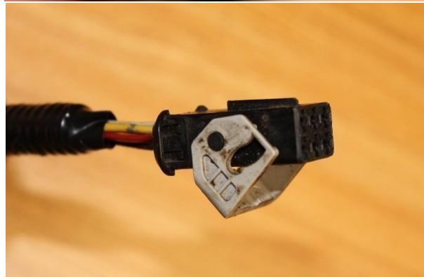
Subaru Six-pin O2 Sensor connector: Just flip the grey bail and pull connectors apart.
