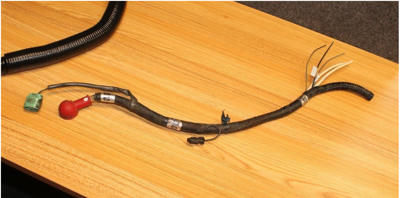
Subaru Alternator Harness: Your harness will have the green and red alternator connectors and the small AC one-wire (multipin in some models) connector.
