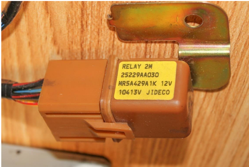
Subaru Main Relay: The vast majority of main relays will look like this. It usually lives near the ECU.
