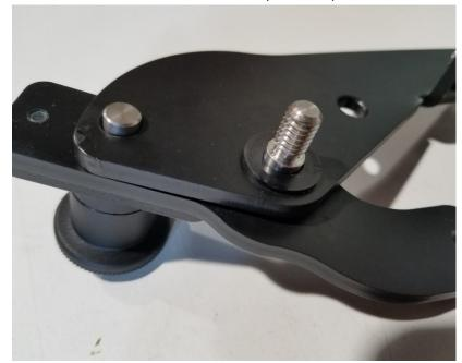
4. Next, install the small curved bracket as shown, followed by a Nylock Nut. Leave the nut loose at this time.
