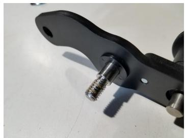
3. Then install the bracket with the bent tab, followed by another plastic washer as shown:
