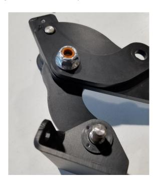
6. Next, you'll install the rubber bumper using the supplied #10-32 bolt and nylock nut. Run the bolt through the bumper, and attach to the bracket as shown.
