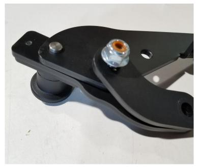
5. Install the rock slider bracket between the other brackets making sure to put a plastic washer between each piece. Also ensure that the bracket is facing the correct direction. Add the last Nylock nut and tighten them both down. Make sure not to over tighten the nuts however. The brackets should be snug but able to move freely:
