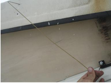
I included the "double-check" using a coat hanger because some pop tops are bowed out more than others - which will throw off the "measure around the outside with a tape" method.
