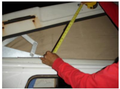
Make a small arc on the pop-top with a pencil at 20 1/4". Now measure up 5  $\frac{3}{4}$ " perpendicularly from the bottom edge of the pop-top, and make a mark where 5  $\frac{3}{4}$  intersects the 20 1/4 arc. These pics were taken on opposite sides of the van.
