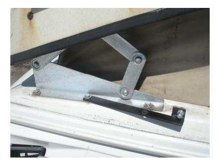
Get the middle bolt finger tight, then remove the front bolt and pivot the front of the bracket into place. Install the longer 10mm bolt (with the washer) and tighten it with your 10mm wrench, also tighten the middle 10mm hinge bolt.
