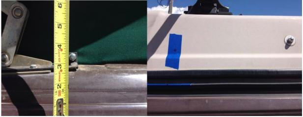
If your ARG mounting hardware is below the line from the lower ball stud to the upper ball stud it will interfere with the strut and you will break the ends of the strut so you will have to flip your hardware, or cut it as short as you can on the inside.
