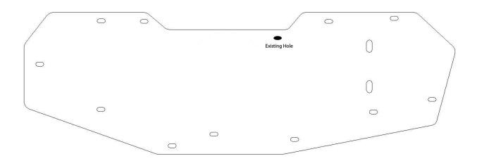
2a. We'll be using the existing hole in the diagram above to mark the additional hole required for the bracket. Align the dipstick tube bracket with the heat shield as shown in the photo using the right-side hole in the bracket aligned with the existing hole.
