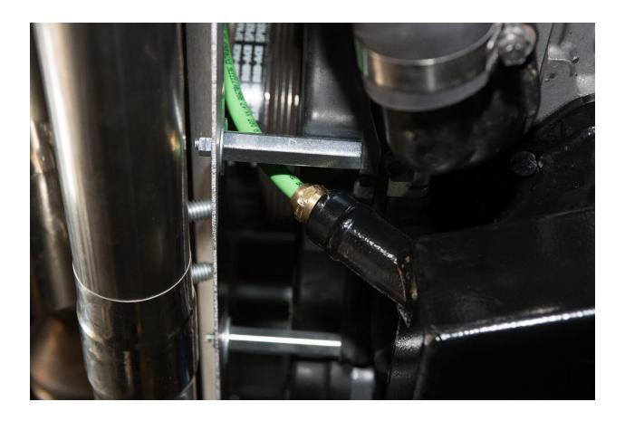
5. Slide the p-clamp over the top of the dipstick in such a way that the flat part of the clamp rests against the heat shield. Insert a bolt from the engine side of the p-clamp and through the bracket and heat shield. Loosely install a washer and nut on the rearside of the heat shield. The dipstick tube will be positioned in between the two bracket mounting bolts. See photo below for reference.
