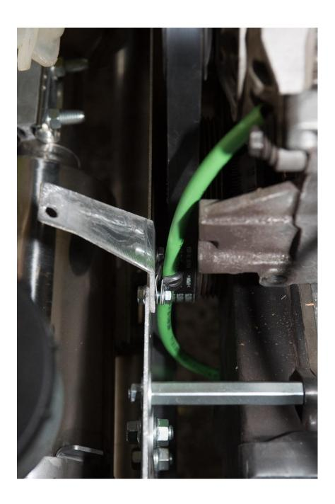
6. Slide the black plastic routing clamp over the dipstick tube so that the bolt hole on the clamp lines up with the bolt hole on the righthand side of the bracket. Insert a bolt through the clamp and bracket and loosely install a nut onto the exposed threads.
