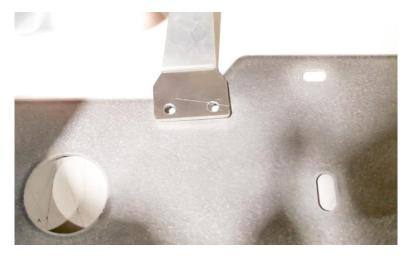
Mark the heat shield through the left hole and remove the bracket. Center punch your mark and carefully drill a new hole with a 1/8" and then a 1/4" bit. Use a file to slot the new hole to match the existing hole.
