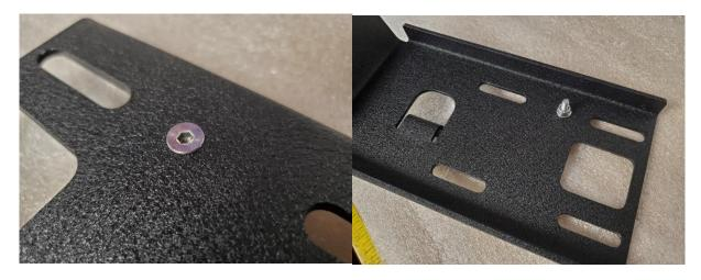
**Step 3:** Now grab the partially assembled lower window bracket (9181) and insert the (3) #10-32 x 5/8" screws and (1) #10-32 x 1" screw from bag B as shown in the image below. (Note: the 1" long screw is shown in the lower RH corner):
