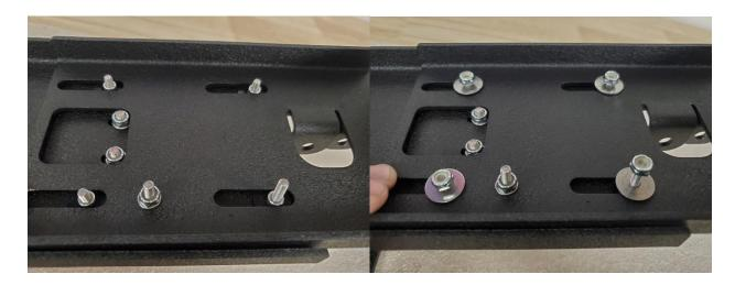
**Step 6:** Lastly, install the small extension spring onto the 1" long screw and the countersunk screw followed by the remaining (2) Nylock nuts. Do not fully tighten these nuts however! Simply tighten until the nylon lock portion can secure the nut to prevent loosening.
