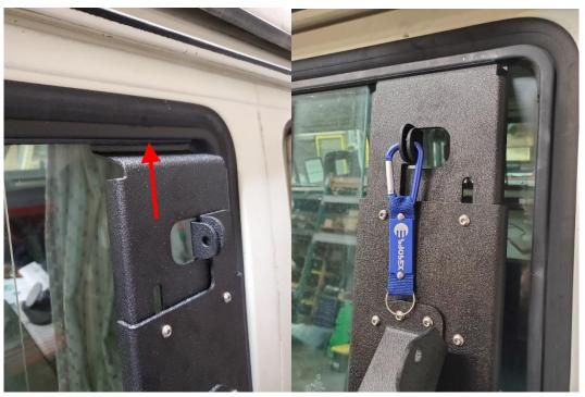
**3.** With the window bracket secured to the van, you can now lift your PS2000 onto the bracket. Use the lock tabs to help visually find center and drop the heater onto the hanger flange. Once, on the bracket, slide the heater to the left so that the lock tabs meet. (Optional: secure the heater to the window bracket via a small padlock).
