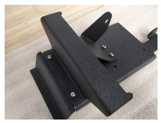
**Step 1 Cont.:** With all four screws in place, go ahead and tighten them using a 1/8" Allen wrench and a 3/8" socket wrench:
