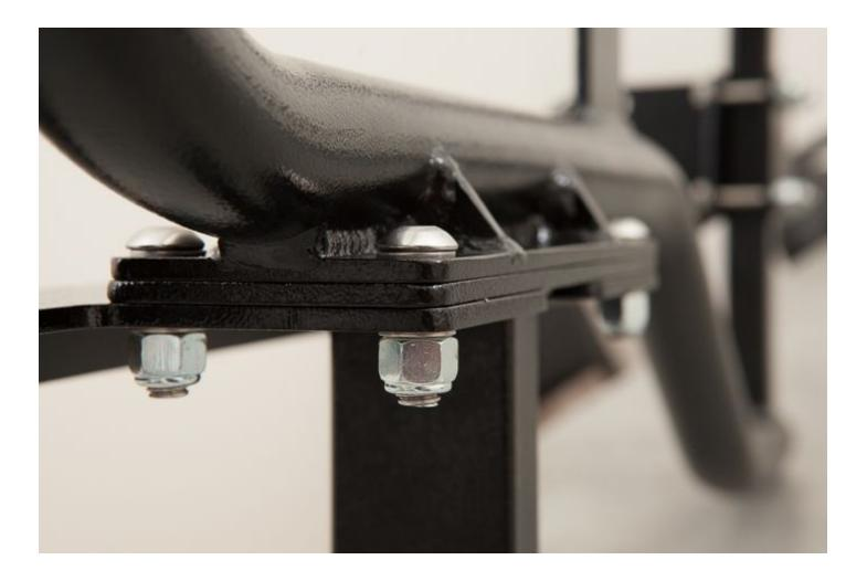
Now onto the far side of the **Shelf Support Frame**. Thread a **8x1.25x50mm LG SS Hex Head Bolt** and **5/16 SS DIN Washer** through the **Shelf Support Frame** and through the **Backing Plate**. Add another **5/16 SS DIN Washer** and finish it off with a **8x1.25 Nylock Nut**. This is to be done at each mounting hole.
