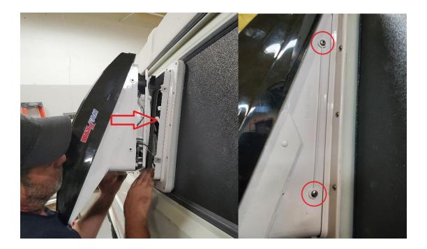
12. To finish up your installation, you can now install the inner garnish trim ring using the four Philips-head screws provided with the fan. Make sure the wiring is on the inside of the ring before tightening the screws as shown below. Tighten the screws by hand only to prevent overtightening.
