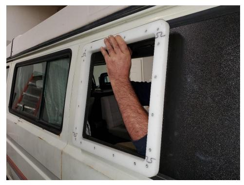
5. Once fully tightened down, carefully wipe any excess silicone off the inside of the flange.
