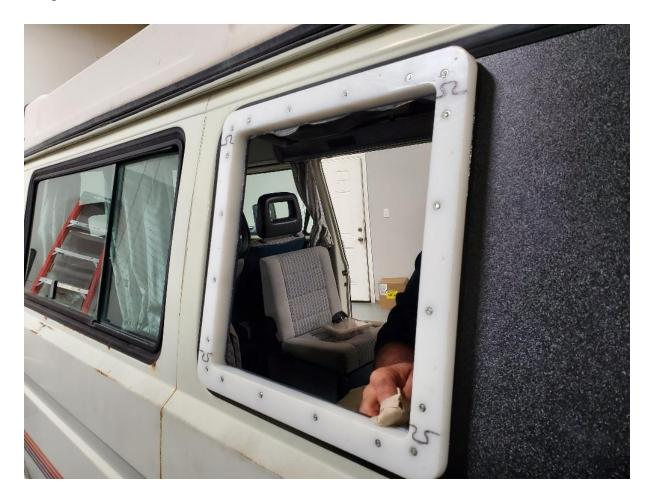
6. Your MaxxFan comes with a piece of plastic trim labeled Interior Garnish Trim Ring that looks like the one below. It is designed to be trimmed down to the thickness of the roof (or in our case, the window fan adapter) in which the fan is going to be installed. Please follow the MaxxFan instructions for best practices for trimming. **Hint:** We recommend letting the garnish trim ring warm up to room temperature to ensure the plastic is not brittle.
