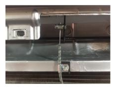
Slip the cable housing mounting clamp around the cable wire and slide it down around the cable housing, so that when it is screwed into place the cable housing lies to the right of the screw, as shown at left. Mount the cable clamp loosely to the clipnut with the last  $\#10 \times 1/2"$  hex-head sheet metal screw. Shift the bellcrank rod left or right so the cable stop nut is vertically aligned with the centerline of the cable.
