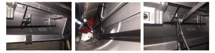
Gently push the bellcrank's cable attachment arm up and down to open and close the door, everything must move freely. Do not bend the bellcrank to force the door closed, instead find out where the drag is and make adjustments as necessary.
