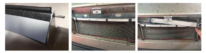
Install three of the (4) clip-nuts over the furthest left, second from left, and furthest right holes in the bottom edge of the cabin air scoop, as shown above center.
