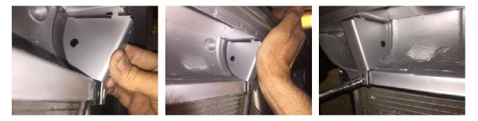
The jamb piece should be held in position where its forward long edge pushes up against and runs along the upper rim of the grille opening, just covering it from below.
