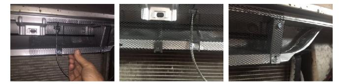
Test inlet door operation again before reinstalling the radiator grille, and the headlights assemblies if they were removed.
