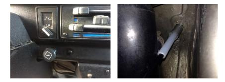
Behind the front grille to the left of the radiator is a <sup>1</sup>/<sub>2</sub>" blind rubber grommet blocking an existing hole in the van firewall. Remove this grommet to expose the hole in the bodywork there that the control cable will go thru (shown at left with poly tube and cable). Insert the poly tube into the hole. You need to maneuver the tube thru the space under the dash until the tube is roughly aligned with the 3/8" hole you drilled.
