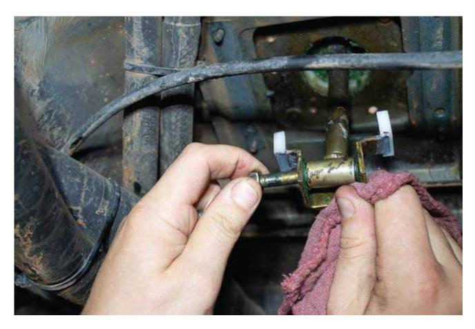
Step 7: Remove the through bolt and set it aside. Remove the small black plastic bushings from the lower hole of the shifter assembly. If you're not replacing them now, you will re-use them in your new Big
