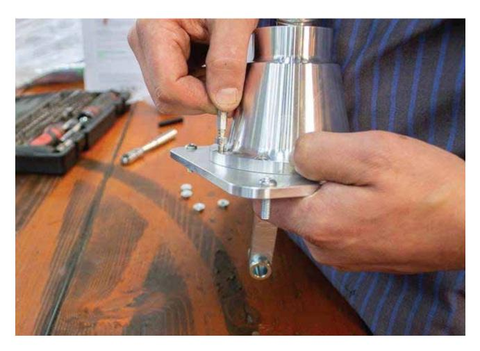
Step 11: Attach the Big Shot Shifter base to the base plate using the remaining hardware.
