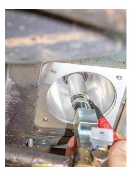
Step 19: With a sharpie, mark the upper shaft and lower block assembly of the Big Shot Shifter V2.0 in a straight line in order to establish orientation. This will help with any adjustments need to make when clocking the shifter shaft for best ergonomic placement.
