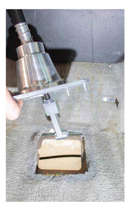
Step 13: Back at the van, align the studs in the bottom of the base plate to the holes in the van floor. Drop the assembled Big Shot Shifter V2.0 into place.
