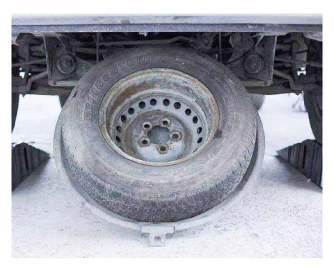
Step 3: Lower the clamshell and remove the spare tire.
