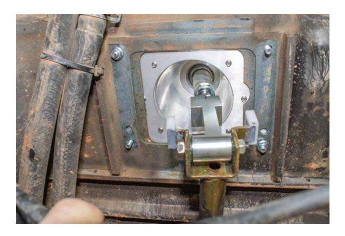
Step 20: Temporarily install two of the lower shift box nuts to the studs coming down through the floor from the Big Shot Shifter base plate.
