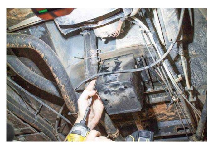
Step 4: Remove the four nuts (10mm) that retain the original shifter assembly to the lower shifter box.
