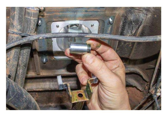
Step 15: Lightly grease the plastic shift rod bushings you removed earlier (or the new ones you purchased from Van Cafe). Insert them into the bottom of the Big Shot Shifter V2.0.
