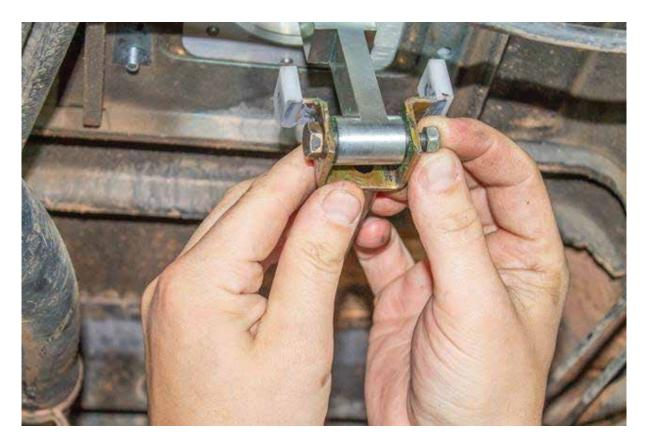
Step 17: Install the nut on the throughbolt.
