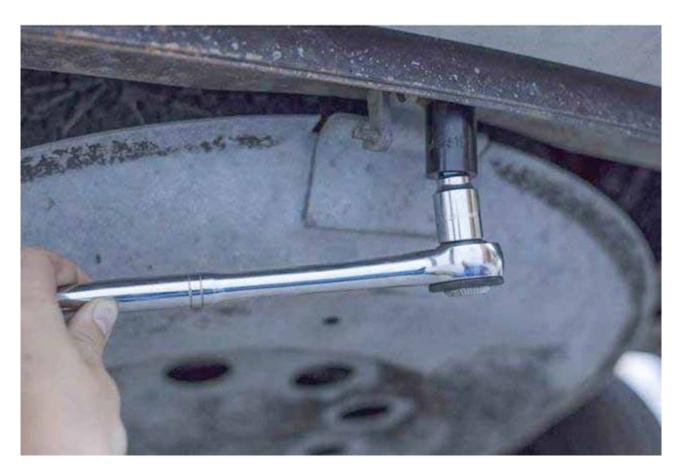
Step 2: Under the front of the van, remove the 19mm bolt that secures your spare tire clamshell.
