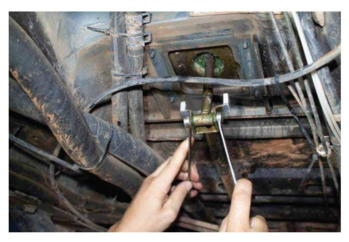
Step 6: Loosen the nut from the through bolt on the shifter assembly to shift rod connection with 10mm and 13mm wrenches.
