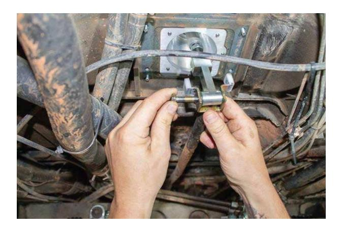
Step 16: Note the orientation of the lower Big Shot Shifter assembly. The larger side of the block and base should be on the passenger-side (right side) of the van. Lightly grease the through bolt and insert it through the shift rod and lower Big Shot Shifter assembly.
