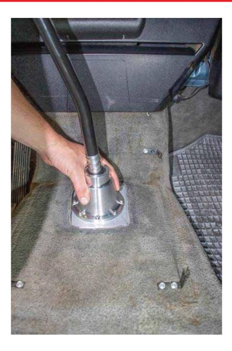
Step 14: With clean hands, lift the carpet over the base plate to hold it while you continue work back under the van.
