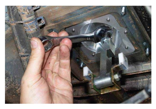
Step 22: Clean your hands and then sit in the driver's seat of the van. Move the shifter shaft around until it is in a comfortable position. You want all gears to be in easy reach from the driver's seat. You may notice the taller height of the Big Shot Shifter V2.0 takes a moment to get acquainted with. You'll come to love not having to reach down for the shift knob.through the shift rod and lower Big Shot Shifter assembly.
