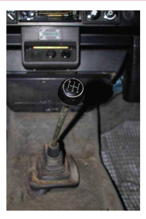
Step 1: Remove the original gear shift knob by twisting counter clockwise. Slide the shift boot up and off the shifter shaft.
