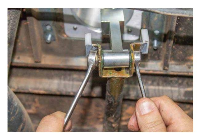
Step 18: Tighten nut and bolt to the shift rod with your 10mm and 13mm wrenches. Note: Overtightening this connection may cause stiff shifting and premature wear of the plastic shift rod bushings.
