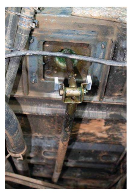
Step 5: Remove the lower shifter box to expose the shift assembly to shift rod connection.
