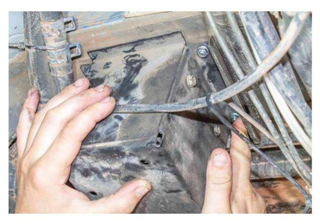
Step 23: Remove the two nuts you temporarily installed holding the base plate from under the van. Grease the tracks inside the lower shift box and the plastic shifter tabs on the shift rod fork. Install the lower shift box using all four nuts.
