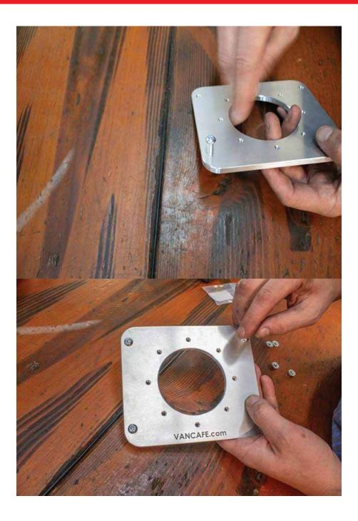
Step 10: Install an M6 x 20 buttonhead screw into each of the four corner holes of the base plate. Run the screws down until snug against the plate.
