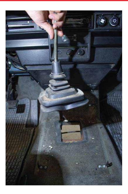
Step 8: From inside the van, carefully lift the original shifter assembly from underneath the carpet. Be careful not to get grease on the interior!
