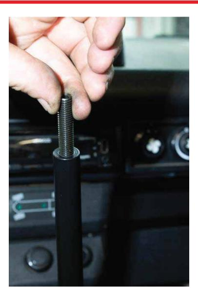
Step 24: With clean hands, install the included stud in the top of the shifter shaft. You will feel it bottom out slightly. It is not necessary to torque this stud as the action of screwing on the shift knob with tighten everything together.
