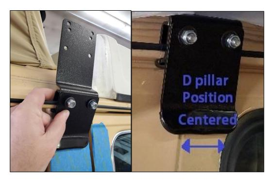
**Step 4:** With the brackets secured to the van, use a small center punch to locate the lower hole in the outer gusset bracket as shown. Then use a ¼" drill bit to drill through the plastic protector and into the Van.
