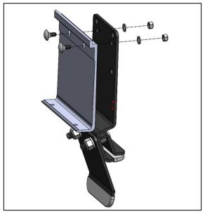
**Step 3:** Next, take the preassembled brackets and slip them over the rain gutter and center them at the B and D pillars. Using one hand, pull the brackets together to take out the slack and tighten both M8 Nylock nuts evenly using a 13mm Socket + ratchet. At this point just tighten the nuts enough to secure the bracket to the van.
