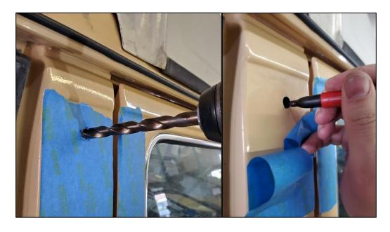
**Step 6:** Utilizing the provided nutsert tool (or a handheld nutsert tool if you have one), install the M6 Nutserts. Hold the brass nut with a 7/16" wrench or set of vice grips and insert the rivet
