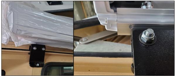
**Front Bracket:** Using a sharpie, put a center mark centered on the mounting bracket, and in the middle of the lower awning channel. Using a 13/64" drill bit carefully drill through all 3 components. **Take your time to prevent drilling into the van!** Deburr the holes and vacuum up any shavings. Using the supplied M5 Phillips head screws, and Nylock nuts, install one into the drilled hole and tighten. This will fully secure the awning to the bracket
