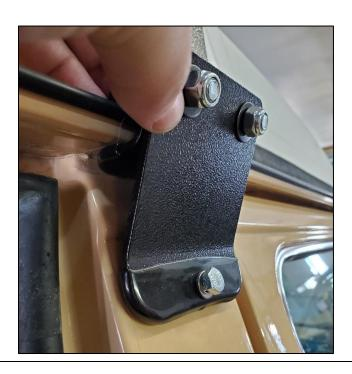
**Step 9: Mounting the Awning (Fiamma)** - With the help of a buddy, carefully lift the awning onto the bracket's channel mount and position the awning so that it is maxed out on the rear mounting bracket. Once you have the awning positioned correctly, go ahead and fully extend the awning and set the legs to support the canvas.
