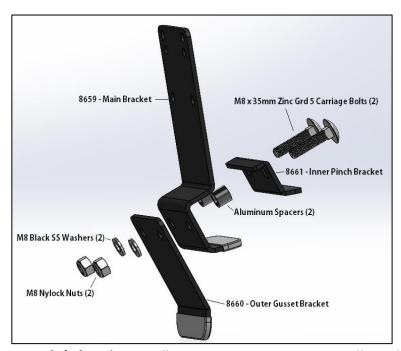
**Step 2.1: (Fiamma Specific)** If you're installing a Fiamma awning, you will need to attach the Fiamma supplied aluminum brackets to the Main Awning Bracket using the supplied M6
