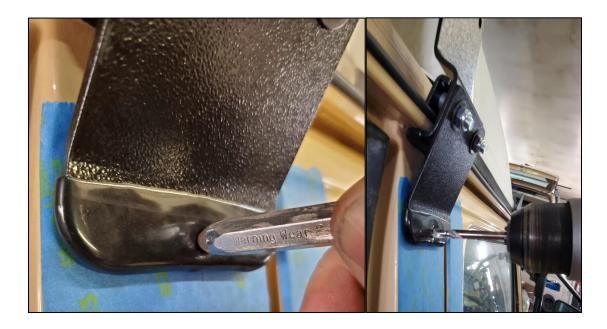
**Step 5:** Next, remove both brackets from the van (leave them assembled if possible) and set them aside. Now using a 25/64" drill bit, enlarge the holes. Carefully deburr the holes and touch up the edges with some paint to prevent corrosion.
