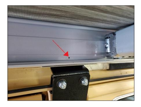
**Rear Bracket:** As for the rear drill location, put a mark centered on the lower channel, and offset to the left of the awning hinge by roughly  $\frac{1}{2}$ ". Repeat the drill process and install the remaining M5 Screw and Nylock nut.
