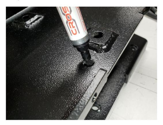
**Step 9:** Once the holes have been touched up, you can now reinstall the winch mount using the (3) 3/8" Bolts, washers and nylock nuts, but leave them hand tight for now.
