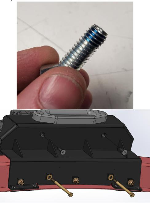
**Step 14:** With the winch fully installed, you can now install the Front and Rear cover plates using the supplied M6 button head bolts, SS washer, Plastic washer and J-Clip nuts (**Bag B**). Install each bolt and simply tighten them down by hand.
