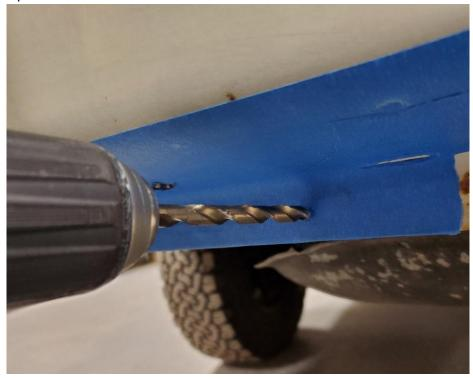
**Step 8:** After all holes are drilled, remove any remaining burrs with a small file or pick. You can also remove the painter's tape and touch up each drilled hole and the winch mount with a paint pen or some paint with a small brush. **TIP:** You may choose to take the time to paint the crash bar black for a nice, muted look.
