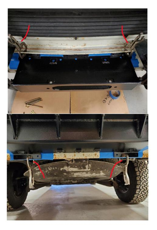
**Step 4:** Once the mount is secured with clamps, drill through the five top and bottom 3/8" mounting holes (Two of which will be the back winch holes). The winch mount will act as a drill guide but try to keep the drill as perpendicular to the surface as possible.
