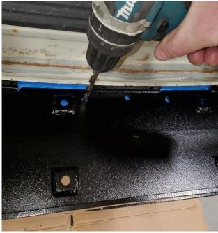
**Step 5:** With all ten 3/8" holes drilled, temporarily install three of the 3/8" bolts with washers and Nylock nuts (**Bag A**). Tighten the bolts down by hand just until there's no visible gaps between the mount and the crash bar. Next, mark the ten small holes using a pen or sharpie.
