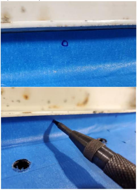
**Step 7:** Using a small drill bit (1/8" or smaller) drill the center of each hole working up to a **5/16"** hole in small steps. Doing so in this way will help prevent any 'bit walk' and keep the hole in the correct position.
