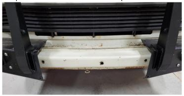
**Step 2:** Using some masking tape, tape the center portion of the crash beam, making sure to cover all areas where the winch mount will contact. This will not only help protect the finish on the winch mount and crash beam but give us a nice contrasting surface for marking the holes.
