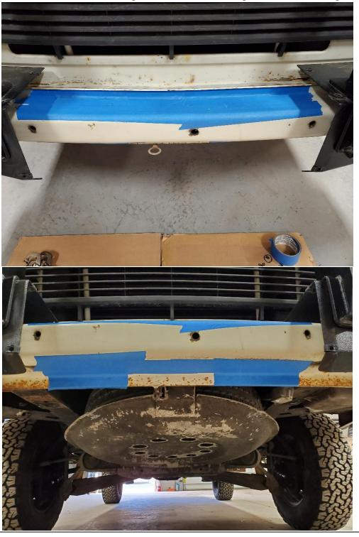
**Step 3:** Install the winch mount onto the van, and center it between the wings. Once centered, use a clamping plier to clamp the mount to the upper pinch weld to prevent it from moving around. **TIP: Temporarily mounting the Front Cover Plate to the wings may help you center the mount on the van.** Use two more clamping pliers to clamp the two lower tabs of the mount to the lower pinch weld. Ensure that the clamps are tight enough to 'suck' the mount to the pinch weld.
