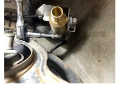
Push the heater hoses onto the valve and take care to position your hose clamps so they can't interfere with the cable and valve actuation lever.
