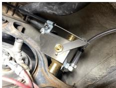
Check the cable adjustment by working the dash lever to open and close the valve a few times, then move the lever hard left as far as it will go. Go below and check that the valve's lever arm is fully closed against its stop. Alter the cable housing position at the valve to adjust as necessary.
