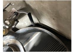
Insert the free end of the bleeder tubing into the guide sleeve from below, and feed it in. The tube will emerge from the guide sleeve at the top and have about 6" free length there.
